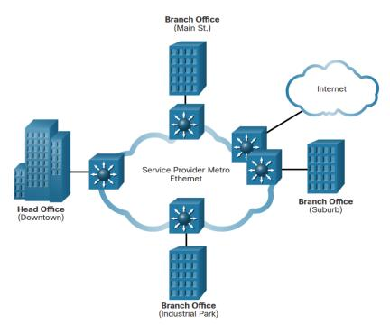
**Note**: Ethernet WANs have gained in popularity and are now commonly being used to replace the traditional serial point-to-point, Frame Relay and ATM WAN links.
