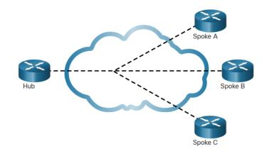
**Note:** The hub router represents a single point of failure. If it fails, interspoke communication also fails.
