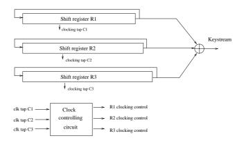
Fig. 1. Schematic description of A5/1
