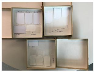
Blood (Martina Marchetti-Deschmann): prepared Sept 19<sup>th</sup> + Oct 4<sup>th</sup>, 2017 Chemical inkjet printer used for printing, 2 square areas: 1+4 dilution with ddH<sub>2</sub>O, 250 μm pitch size, 5x5 mm , 240 pL/spot; additionally a blood spot prepared with a pipette - 0.5 μL undiluted blood Exemplary sample set:
