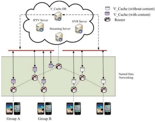
Figure 2. System Architecture of N-Screen ShopMark
