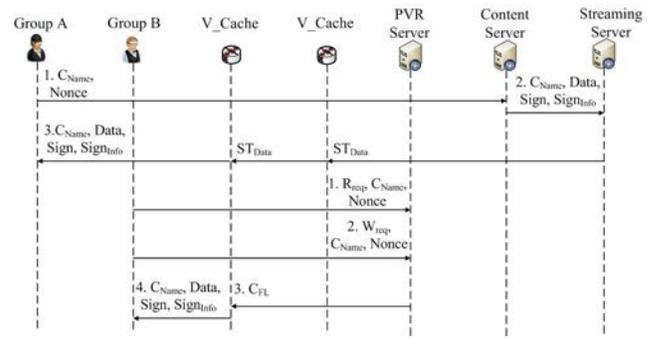
Figure 3. System Architecture of N-Screen ShopMark
