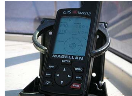
Civilian GPS receiver ("GPS navigation device") in a marine application.
