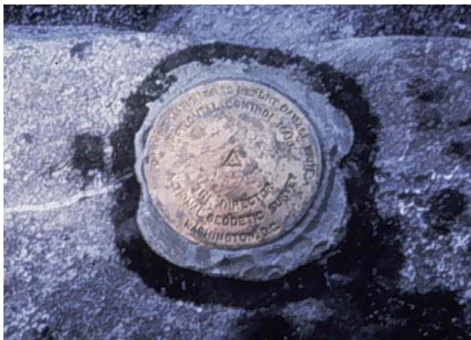
Figure 2.16.1 In the U.S., high-order horizontal control point locations are marked with permanent metal "monuments" like the one shown above. The physical manifestation of datum is a network of control point measurements.
