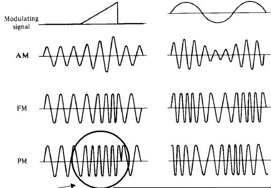
Constant frequency follows constant modulation waveform derivative
