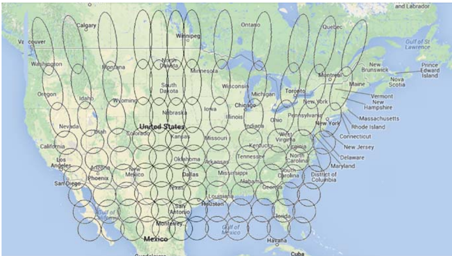
Figure 3.6 Spot-beam operation of a HTS (typical because of antenna distortion).
