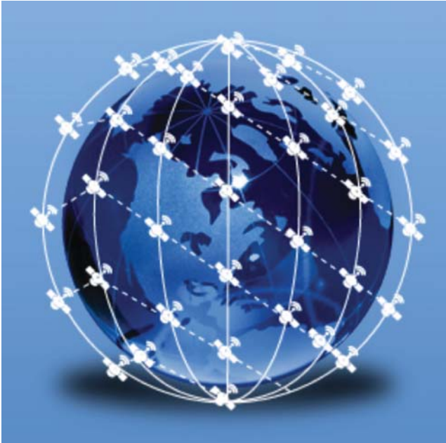
Figure 6.17 Iridium global constellation of 66 cross-linked low earth orbit (LEO) satellites.
