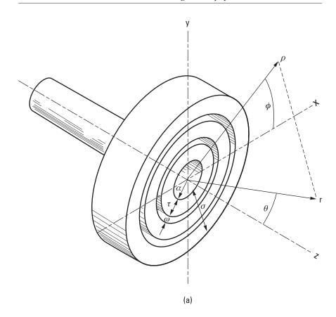
Figure 7.16 Compact circular flanged horn with annular slots cut into the waveguide. The slots are used to shape the pattern and reduce sidelobes. (Reference [9], with permission.)
