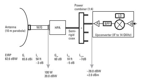
Figure 7.4 Uplink gain budget for an earth station high-power transmit chain (assumed to be at 18.2 GHz).
