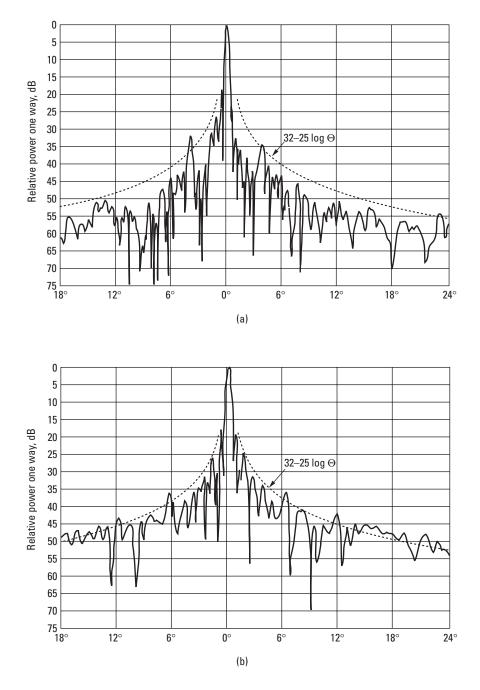
Figure 7.27 Measured 10-m earth station antenna pattern at C band: (a) transmit, 6,175 MHz, (b) receive, 3,950 MHz.
