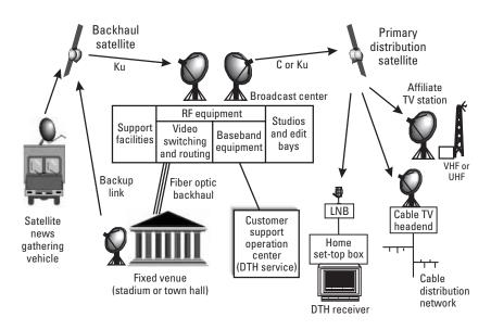
Figure 5.1 Combined satellite TV network, used to acquire real-time programming and distribute to TV stations, cable TV systems, and DTH receivers.
