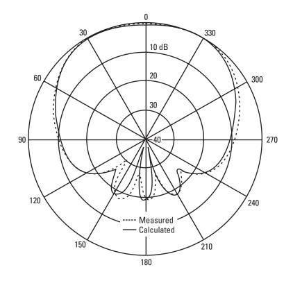
Figure 7.7 Broad beam pattern of a rectangular microstrip patch MSS antenna.
