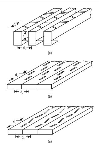
Figure 7.18 Waveguide slot arrays: (a) edge slot array; (b) displaced longitudinal slot array; (c) inclined series slot array. (Reference [9], with permission.)
