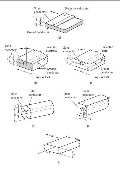
Figure 7.11 Microwave transmission lines: (a) microstrip line, (b) triplate stripline, (c) suspended stripline, (d) circular coaxial line, (e) square coaxial line (squarax), and (f) rectangular waveguide.
