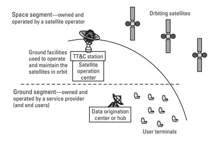
Figure 1.1 Definition of the space segment and the ground segment.
