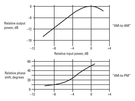
Figure 8.5 TWT nonlinear characteristics (AM-to-AM and AM-to-PM).
