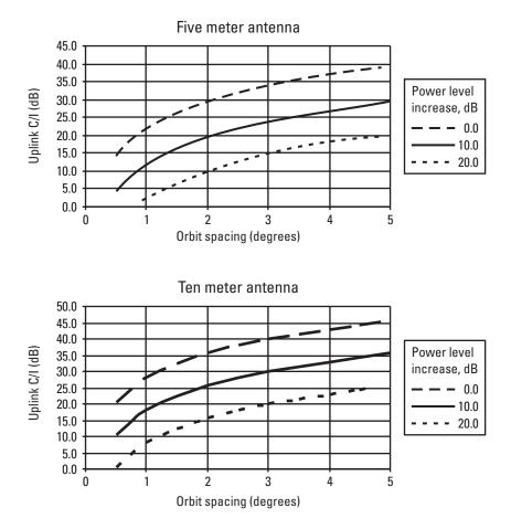
Figure 3.6 Uplink C/I due to a C-band transmitting earth station for either 5-m or 10-m reflector diameter, as a function of orbit spacing and uplink power level increase (assumes 10% increase in offset angle due to ground geometry).
