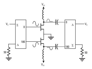
Figure 9.9 Push-pull Class B RF amplifier using a pair of microwave FET amplifier modules and two 180° hybrids.
