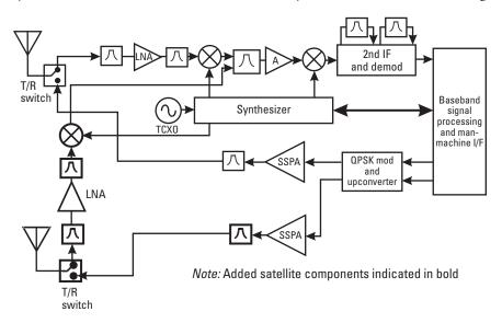
Figure 9.20 Modifications to the design of a standard GSM mobile phone to accommodate a satellite GMPCS mode of operation.
