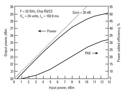
Figure 9.12 Power-frequency response of the packaged MMIC chip. (Reference [2], with permission.)
