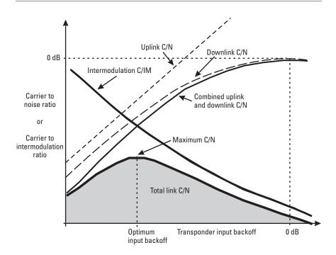
Figure 8.2 Tradeoff between C/N and C/IM in an FDMA transponder or HPA.
