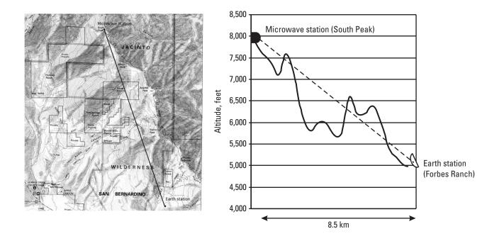
Figure 10.6 Example of an interference path study for a mountaintop microwave station and a well-shielded earth station antenna.
