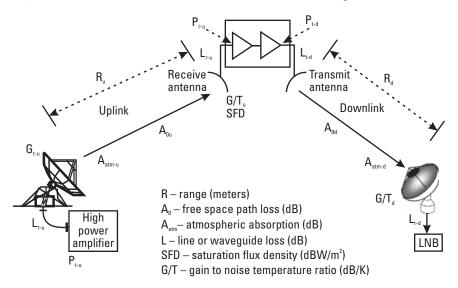
Figure 2.3 Key elements and terms for the uplink and downlink.
