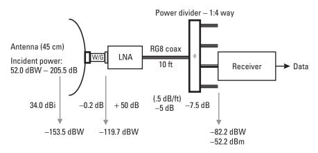
Figure 7.10 Typical receiving chain gain budget at 12 GHz.
