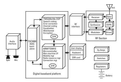
Figure 9.19 Block diagram of generic handheld mobile phone, based on application of ASIC and programmable DSP components.
