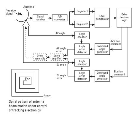
Figure 7.24 Block diagram of a step track system, which detects changes in received power and moves the beam according to an inward spiral pattern.
