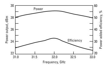
Figure 9.13 Output power and efficiency of the packaged MMIC chip at 32 GHz. (Reference [2], with permission.)
