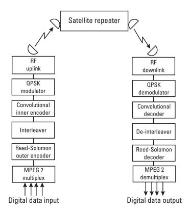
Figure 3.2 Simplified end-to-end block diagram for a DVB MPEG-2 link.
