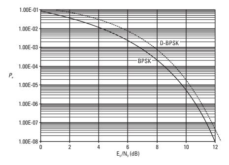
Figure 2.9 Theoretical probability of bit error (P<sub>e</sub>) for BPSK and differential BPSK.
