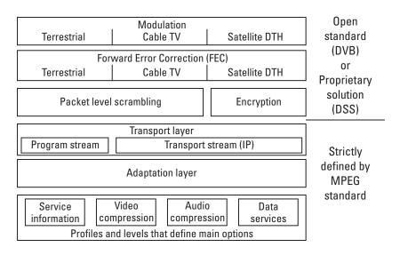
Figure 5.2 Structure of MPEG-2, indicating its protocol stack and support for satellite and terrestrial broadcasting networks (reference: http://www-it.et.tudelftnl).
