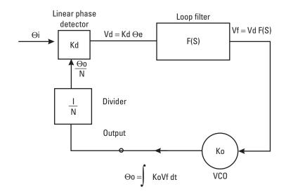
Figure 8.8 Basic phase-lock loop feedback system.
