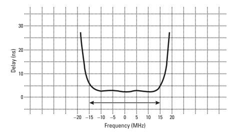
Figure 8.4 Typical group delay characteristic (delay versus frequency).
