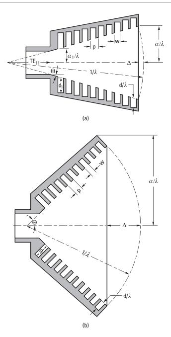
**Figure 7.15** Cross-section view of corrugated horn showing usual slot configuration for (a)  $\theta$  small, and (b)  $\theta$  large. This design offers a symmetrical pattern with low sidelobes and high efficiency. (Reference [9], with permission.)
