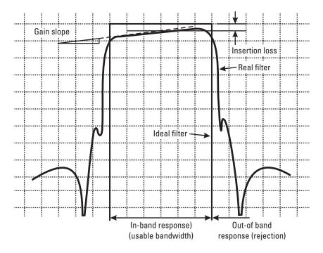
Figure 8.3 Ideal and real filter amplitude responses (gain versus frequency).
