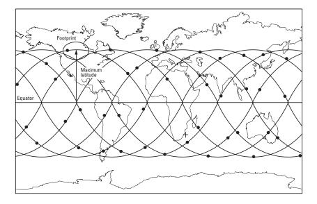
Figure 8.9 Ground track for a LEO constellation as presented by Satellite Tool Kit (image courtesy of Analytical Graphics, Inc.).
