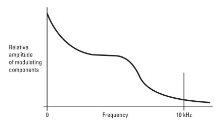
Figure 8.6 Spectrum of a signal that would, if frequency-modulating a carrier, result in typical short-term frequency instability.
