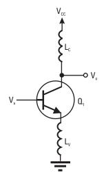
Figure 9.8 Basic Class A RF amplifier using a junction transistor.
