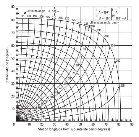
Figure 3.5 Ground antenna elevation angle and azimuth to a GEO satellite.
