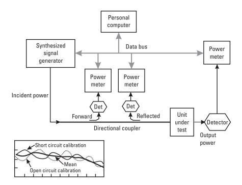
Figure 11.4 Amplitude-frequency response measurement system, using a synthesized signal generator as the input to the unit under test (UUT).
