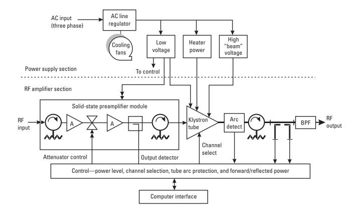
Figure 7.34 Generalized block diagram of a high-power klystron power amplifier.
