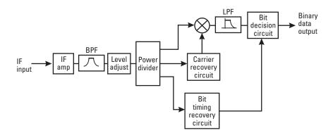
Figure 2.8 Simplified BPSK demodulator block diagram.
