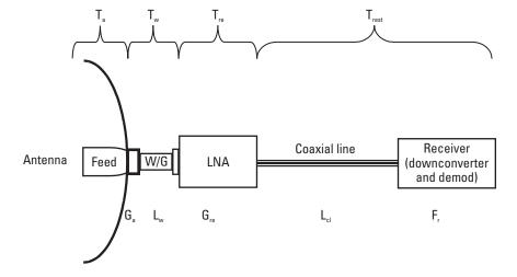
Figure 7.9 Typical block diagram to determine receiving system noise temperature.
