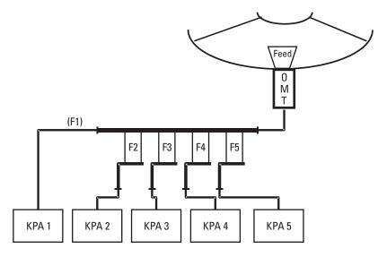
Figure 7.29 A high-power RF multiplexer used to combine the outputs of several klystron power amplifiers in an earth station.
