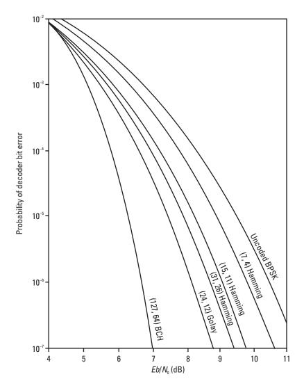
Figure 6.10 Block code performance (reprinted with permission of Prentice Hall, Englewood Cliffs, N.J.).
