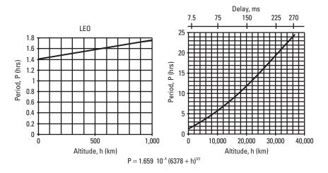
Figure 3.1 Orbit period and propagation delay for various satellite altitudes, based on Kepler's third law of planetary motion.
