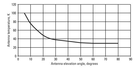
Figure 7.6 Typical antenna temperature contribution with elevation angle.
