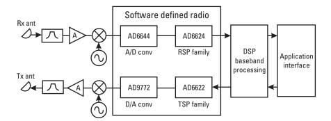
Figure 9.15 Software-defined radios combine the functionality of A/D conversion, receive signal processing (RSP), transmit signal processing (TSP), and D/A conversion.
