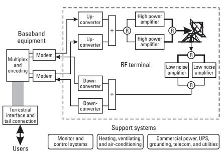
Figure 2.1 Operating elements of a major earth station, including RF terminal, baseband equipment, terrestrial interface and tail connection, and support systems.
