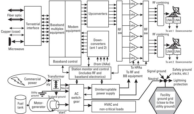
Figure 10.1 General arrangement for a major earth station and its supporting facility, indicating information flow and critical connections.
