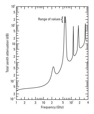
Figure 2.4 Typical atmospheric absorption (dB).
