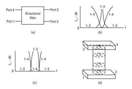
Figure 7.30 Characteristics of an RF directional filter: (a) schematic diagram, (b) transfer characteristic of single cavity, (c) characteristic of multiple cavity, (d) drawing of multiple cavity directional filter.
