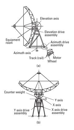
Figure 7.22 Antenna mount and drive configurations: (a) azimuth-elevation, (b) X-Y.
