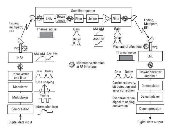
Figure 8.1 Signal impairment contributions in a typical end-to-end satellite link.
