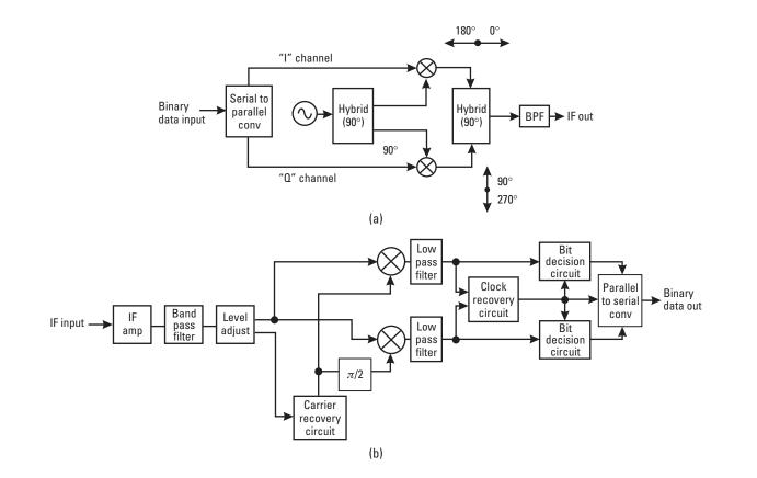
Figure 6.7 Generalized block diagram of a QPSK (a) modulator and (b) demodulator.
