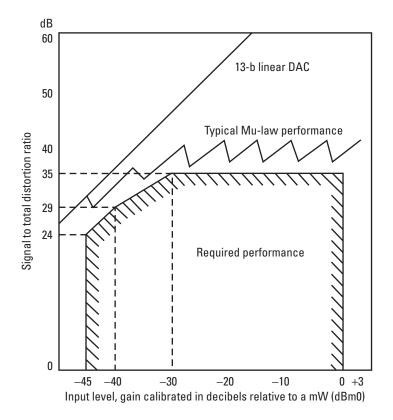
Figure 4.5 Signal-to-quantization distortion performance for Mu-law companded and 13-bit linear digital-to-analog conversion as compared with telephone network requirements. (Same attribute as Figure 4.3) Reference [2], with permission.
