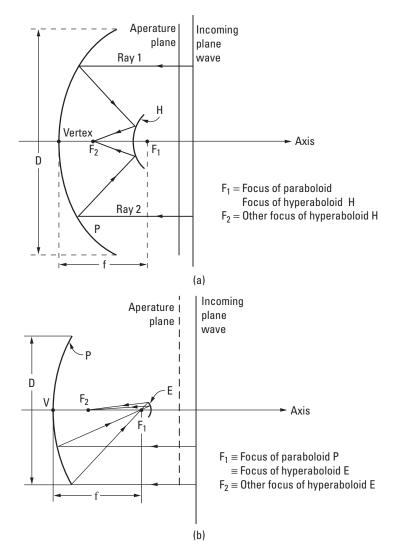
Figure 7.20 Geometry of the reflector and subreflector in an earth station antenna: (a) Cassegrain geometry, (b) Gregorian geometry.
