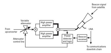
Figure 7.3 Closed-loop uplink power control system, using a dedicated satellite UPC beacon.
