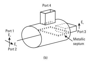
Figure 9.3 Arrangement of an OMT used to combine transmit and receive in the same feed: (a) illustration, (b) drawing.
