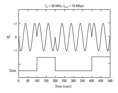
Figure 2.6 BPSK time domain waveforms.
