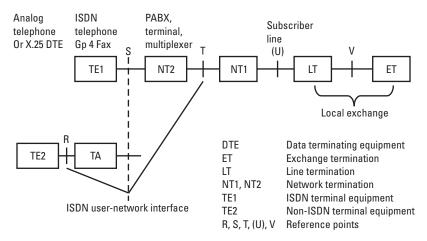
Figure 4.6 Standard user interface definitions for narrow-band ISDN.
