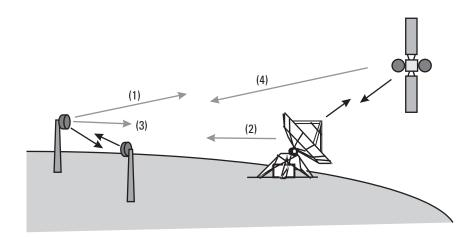
Figure 10.4 Interference potential between satellite links and terrestrial microwave links that use the same frequency band. Paths 2 and 3 are of direct concern in terrestrial coordination; paths 1 and 4 are covered in the radio regulations of the ITU.
