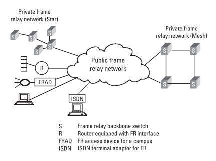
Figure 4.13 Implementation of Frame Relay.
