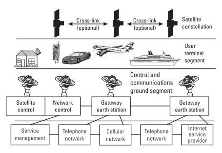
Figure 6.1 Main architectural elements of a communications ground segment (fixed or mobile).
