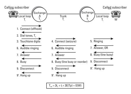
Figure 4.8 Telephone call signaling sequence, indicating transmission nodes, time duration, and delays.
