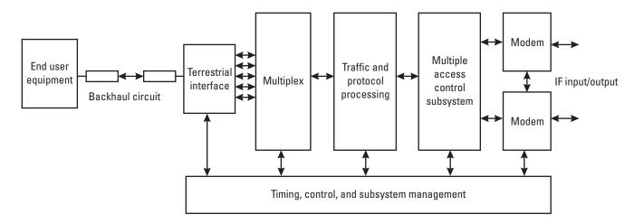
**Figure 6.5** Baseband subsystem of a central hub earth station for digital communications services.
