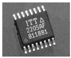
Three-stage MESFET 1800 to 2000 MHz (PCS, DECT, and WLL) 0.5 W output, 29.3 dB gain 49% power added efficiency
