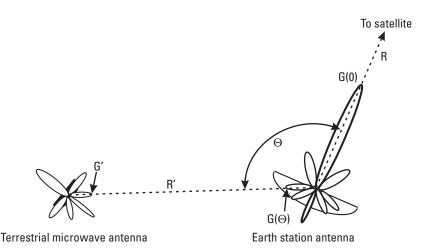
Figure 10.5 Interference geometry (top view) for terrestrial interference to reception at an earth station with a large-diameter antenna.
