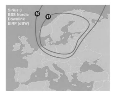
Figure 3.3 Sirius 3 BSS Nordic coverage from 5.0° east longitude, indicating EIRP performance at the 52 dBW level (illustration courtesy of NSAB).
