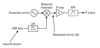
Figure 2.7 Simplified BPSK modulator block diagram.
