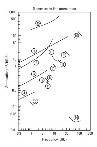
Figure 7.5 Attenuation characteristics of typical coaxial and waveguide transmission lines.
