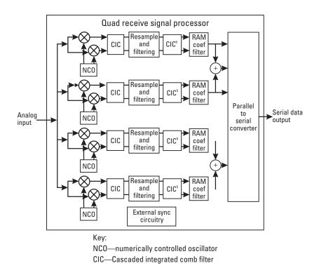
Figure 9.16 In a software-defined radio, the receive signal processor (RSP) is designed to replace an LO, quadrature mixer, channel filter, and data decimator.
