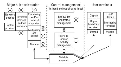
Figure 6.4 Generic baseband architecture for a digital communications satellite network.
