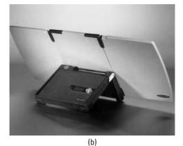
Figure 1.8 Examples of compact MSS user terminals for use in the Inmarsat system: (a) Standard M; (b) Standard M4 (photos courtesy of NERA).
