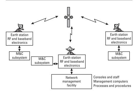
Figure 11.1 Modern satellite network management system.
