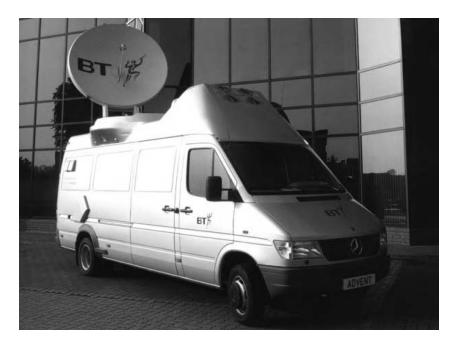
Figure 7.26 Transportable/mobile video uplink antenna system (photo courtesy of Advent Communications).
