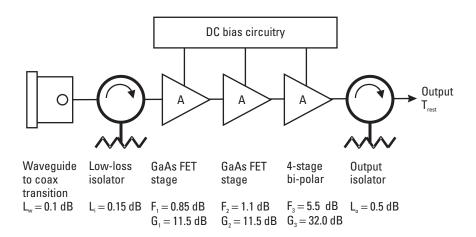
Figure 7.8 Low noise amplifier (LNA) block diagram, showing a waveguide-to-coax adaptor input, a three-port coax isolator, and three stages of amplification. The isolator at the output reduces interaction with downstream components.
