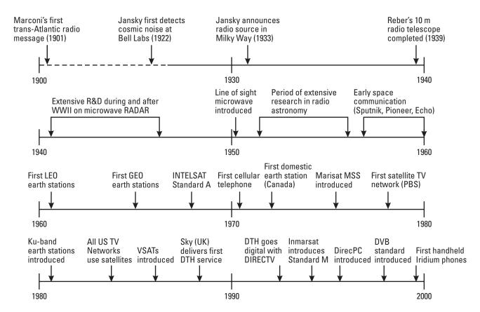
Figure 1.2 Overall timeline of ground segment and earth station development.
