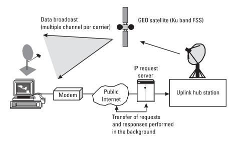
Figure 5.4 Architecture for IP data broadcasting and return channel via PSTN.
