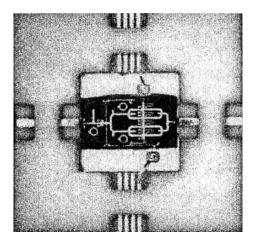
Two stages with output stage containing four GaAs transistors in series bias, 31 to 33 GHz (Ka band uplink) 800 mW maximum output at 24 VDC 32 to 35% power added efficiency
