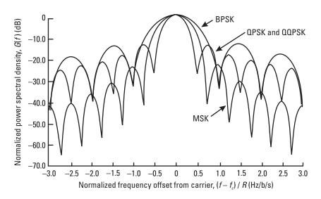
Figure 6.8 Normalized power spectral density for BPSK, QPSK, OPSK, and MSK.
