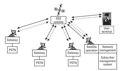
Figure 4.1 GEO mobile satellite and network architecture.
