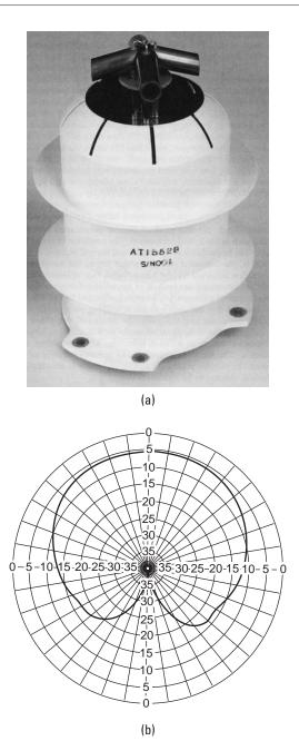
Figure 9.5 Illustration (a) and performance (b) of a drooping-dipole antenna with crossed elements to achieve circular polarization and symmetrical coverage of the sky.
