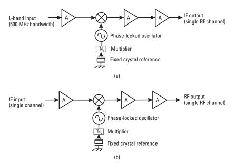
Figure 7.35 Block diagrams of fixed-frequency converters used in earth stations: (a) up converter, (b) down converter.
