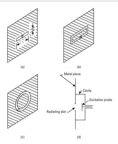
Figure 7.17 Slot antenna elements: (a) rectangular, (b) folded rectangular, (c) annular slot, and (d) cavity backed slot. (Reference [9], with permission.)
