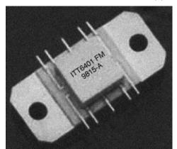
Two-stage GaAs MMIC 4.5 to 7.1 GHz 2.5 W output, 18 dB linear gain 40% power added efficiency 43 dBm third order intercept
