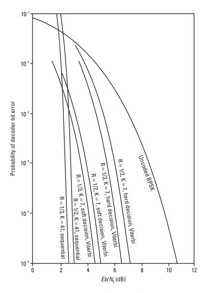
Figure 6.9 Convolutional code performance (Source: IEEE).
