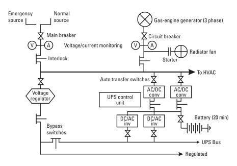
Figure 10.2 Simplified installation diagram for a power system incorporating dual utility feeds, a standby motor generator, and an uninterruptible power supply.
