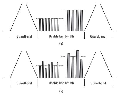
Figure 7.1 A multicarrier transponder: (a) with carriers aligned properly in power; and (b) with excessive power variations that degrade service for some and reduce the total backoff.
