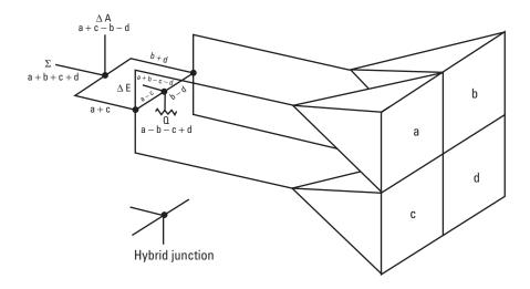
Figure 7.25 Simple two-axis monopulse feed.
