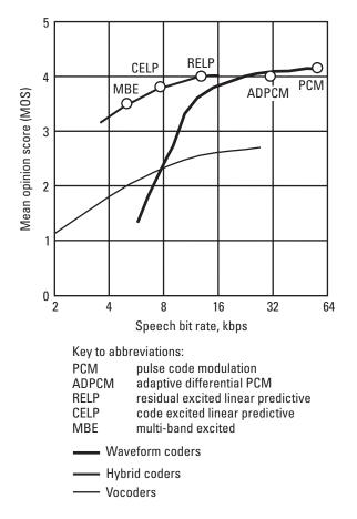
Figure 4.7 Comparison of bit rate and MOS for various digital speech compression techniques.
