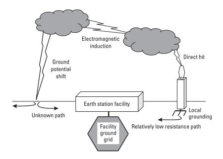
Figure 10.3 Direct and indirect paths for lightning to reach the interior of an earth station.
