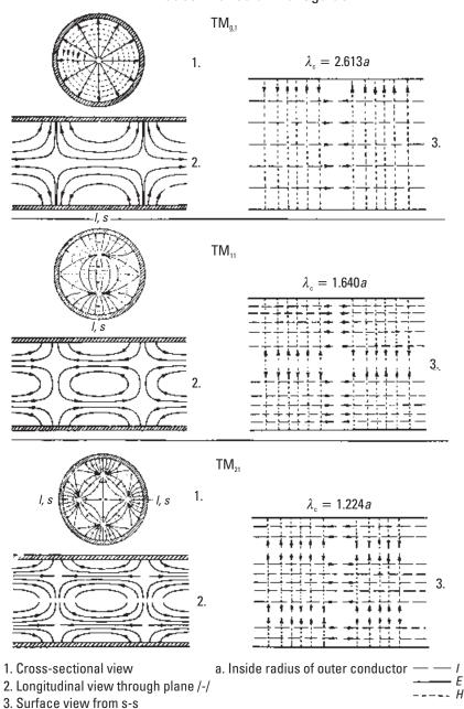
TM modes in circular waveguide
