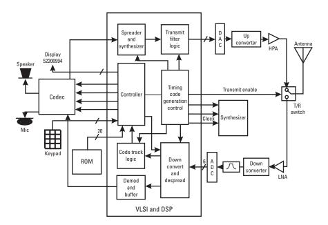
Figure 9.14 Wireless digital user terminal employing a spread-spectrum receiver.
