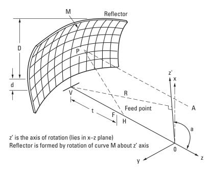
Figure 7.21 Multibeam torus antenna geometry.
