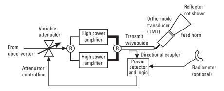
Figure 7.2 Open-loop uplink power control system, using an optional RF radiometer to detect rain attenuation from the ground.
