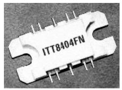
Two-stage GaAs MMIC 5.5 to 7.0 GHz 5 W output, 18 dB linear gain 25% power added efficiency
