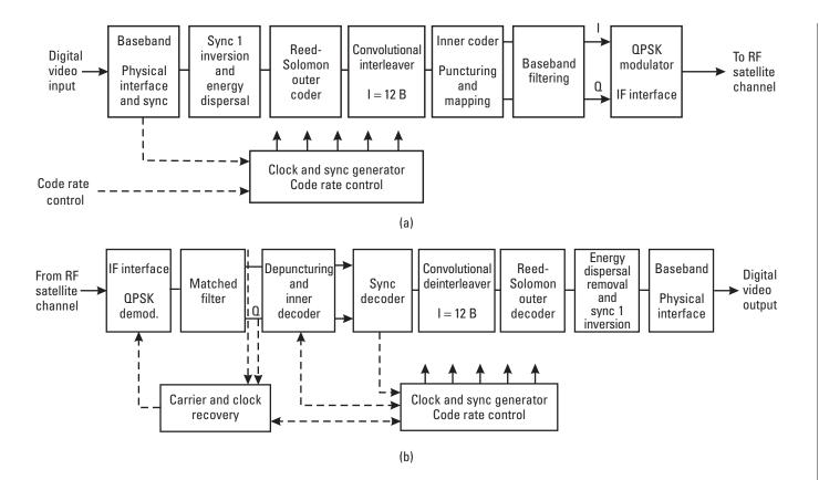
Figure 5.3 Functional block diagrams of the DVB-S (a) transmitter and (b) receiver.
