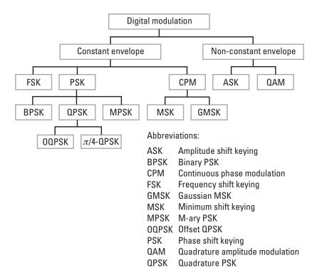
Figure 6.6 Digital modulation tree, indicating the primary techniques used in commercial satellite communications.
