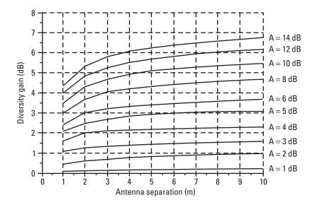
Figure 5.7 Diversity gain versus antenna separation distance for a family of single antenna fade levels, based on rural roadside tree measurement campaigns [10].
