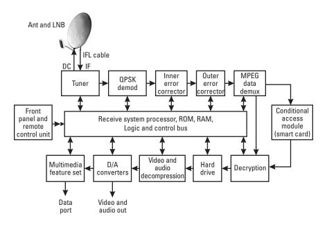
Figure 9.17 Generic block diagram of a digital direct-to-home integrated receiverdecoder (MPEG-2).
