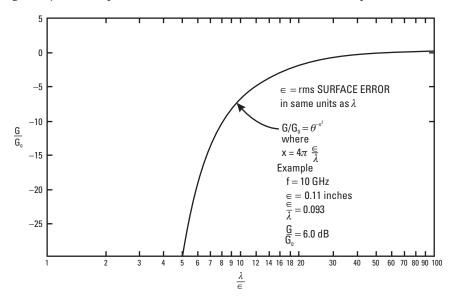
Figure 7.28 Normalized loss due to finite surface error (according to Ruze).
