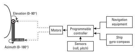
Figure 7.23 Functional block diagram of a program tracking system for a limited motion reflector antenna installed on a ship.
