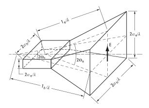
**Figure 7.14** Configuration and dimensions for a smooth-walled pyramidal horn. The radiation pattern can be adjusted with the values of  $\theta_e$  and  $\theta_n$ . (Refence [9], with permission.)
