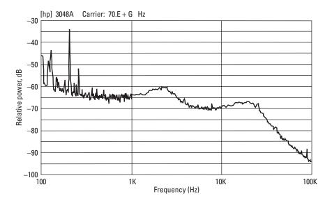
Figure 8.7 Phase noise sideband profile for a downconverted continuous wave tone generated by a 14.5-GHz VSAT terminal.
