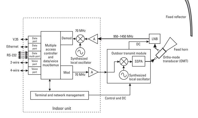
Figure 9.1 Block diagram of typical two-way VSAT for fixed satellite communications.
