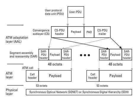
Figure 4.12 The protocol layers and cell structure of ATM.
