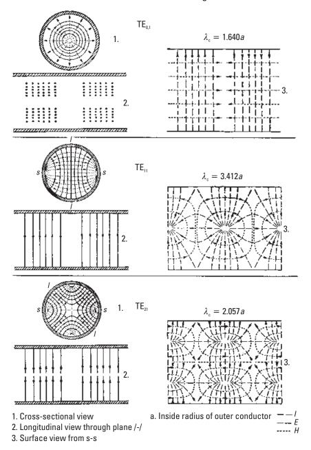
Figure 7.13(a) Propagation modes in circular waveguide: TE modes.
