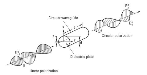
Figure 7.19 Conversion from linear to circular polarization by a 90° polarizer consisting of a dielectric plate.
