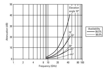
Figure 2.5 Rain attenuation versus frequency for 99.5% and 98% availability in a temperate climate.
