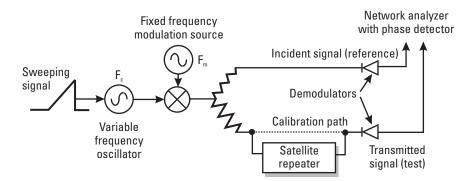
Figure 11.5 Dynamic measurement of group delay, using a modulated signal that counters the effects of frequency translation and Doppler due to a satellite repeater.
