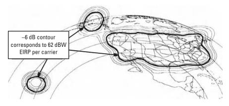
Figure 5.5 Coverage footprint of WorldSpace "XM Radio" DAR satellite at 115° west longitude (filing before the FCC).
