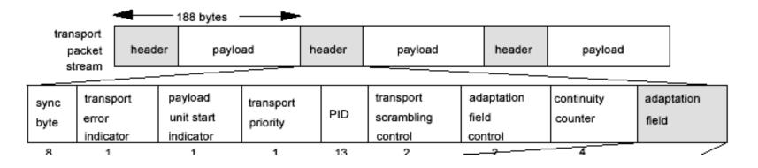
Sync byte – always hex 47 (bin 1000 1111) Transport error – error during transport Payload start (PES or PSI data) Transport priority PID (13 bits : dec value 0-8192, hex 0-1FFF) Transport scrambling (only payload): 0 or 1,2,3 Adaption: 1: P, 2: A, 3: A, P Continuity pointer: Increases modulo per PID basis
