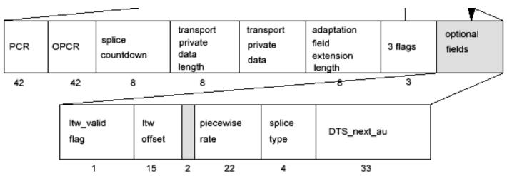
Program clock reference – intended time of arrival Spliced – signed counter for splicing Private data length – up to transport Extenstion length
