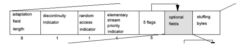
Field length Discontinuity indicator Random access indicator – helps random access Elementary stream priority (e.g. Video Intracoded slice) Stuffing bytes – fill the transport packet to 188 bytes
