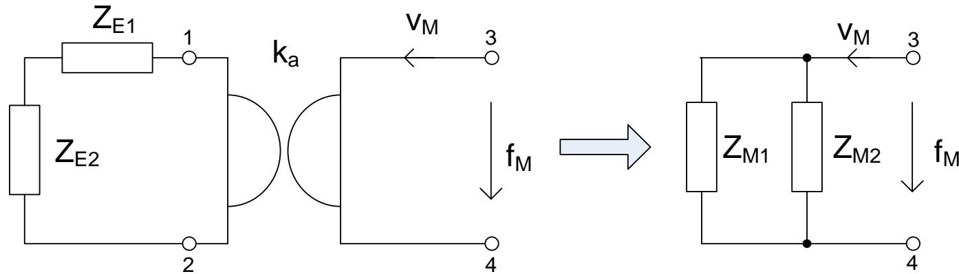
$$Z_E = Z_{E1} + Z_{E2} \Rightarrow \frac{1}{Z_M} = \frac{Z_E}{k_a^2} = \frac{Z_{E1} + Z_{E2}}{k_a^2} = \frac{Z_{E1}}{k_a^2} + \frac{Z_{E2}}{k_a^2} = \frac{1}{Z_{M1}} + \frac{1}{Z_{M2}}$$
