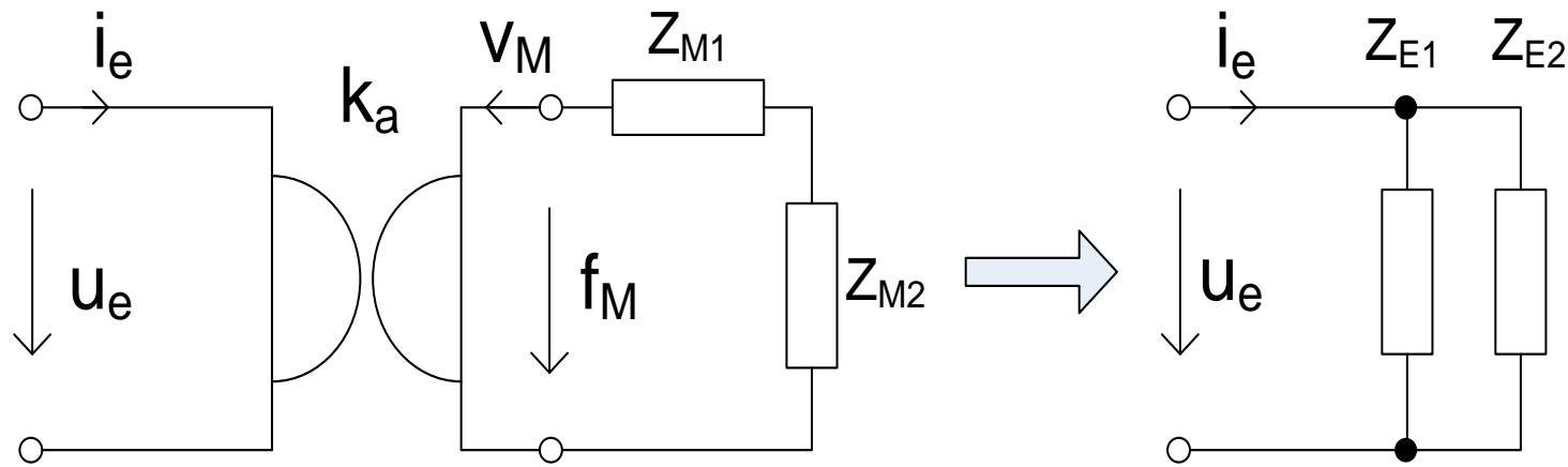
$$Z_M \cdot Z_E = k_a^2 : \text{ ak } Z_M = Z_{M1} + Z_{M2} \Rightarrow \frac{1}{Z_E} = \frac{Z_{M1} + Z_{M2}}{k_a^2} = \frac{Z_{M1}}{k_a^2} + \frac{Z_{M2}}{k_a^2} = \frac{1}{Z_{E1}} + \frac{1}{Z_{E2}}$$
