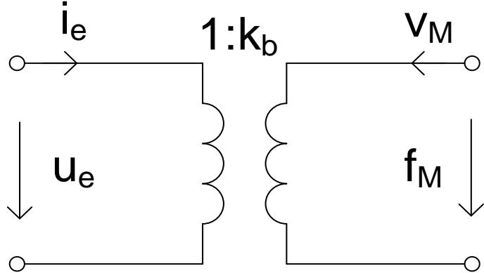
$$\begin{aligned} f_M &= k_b \cdot u_e' + 0 \cdot i_e' \\ v_M' &= 0 \cdot u_e' + k_b^{-1} \cdot i_e' \end{aligned}$$
