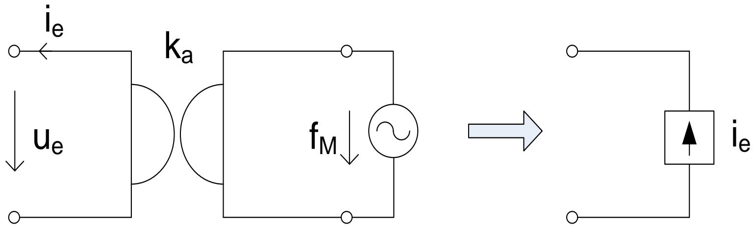
$$f_M = k_a i_e \quad \Rightarrow \quad i_e = \frac{f_M}{k_a}$$
