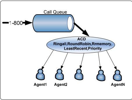
Figure 1-12 Asterisk as a Contact Center Platform
