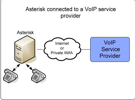
Figure 7.8 Asterisk connected to a VoIP service provider
