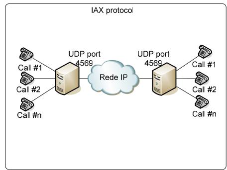
Figure 6.2: Multiple calls over a single UDP connection
