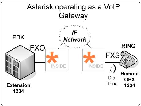
Figure 4.3 Asterisk operating as a VoIP gateway
