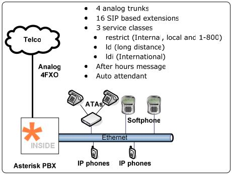
Figure 9.19 Complete PBX example
