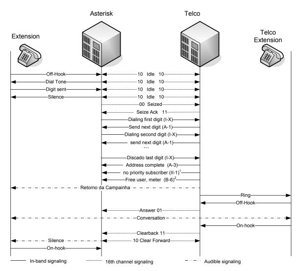
The sequence above illustrates a call originating from an Asterisk's extension to a terminal in the PSTN. The PSTN drops the call and ends the communication.
