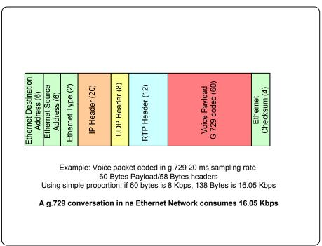
Figure 5.11 increasing the voice payload to reduce bandwidth
