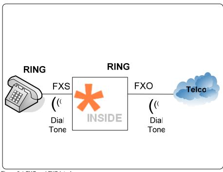
Figure 3.1 FXO end FXS Interfaces
