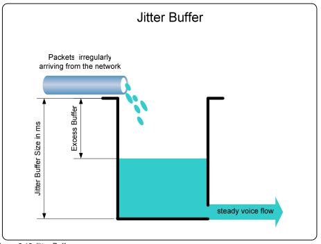
Figure 6.10 Jitter Buffer
