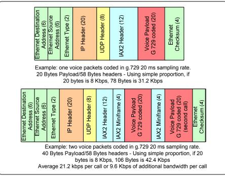
Figure 5.11 IAX2 trunk mode bandwidth reduction
