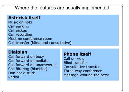
Figure 10.2 where the features are implemented
