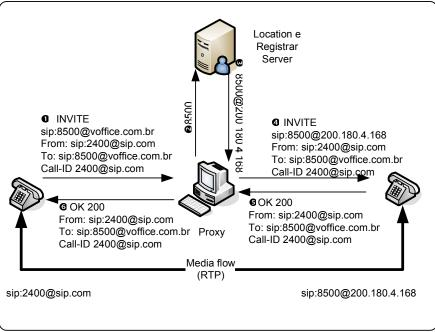
Figure 7.4 SIP proxy Operation
