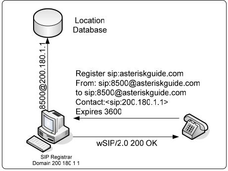
Figure 7.3 SIP Register Process
