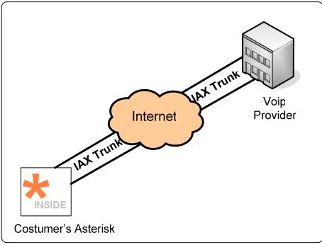
Figure 6.5 Connecting to a VoIP Provider
