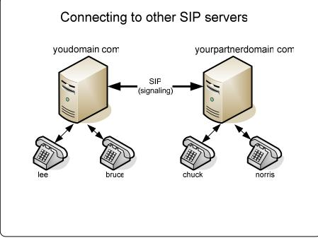
Figure 7.10 connecting other users using a SIP URI.
