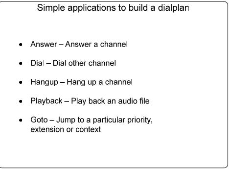
Figure 8.6 Simple applications to build a dialplan
