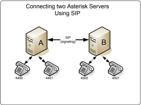
Figure 7.9 Connecting two asterisk server together using SIP
