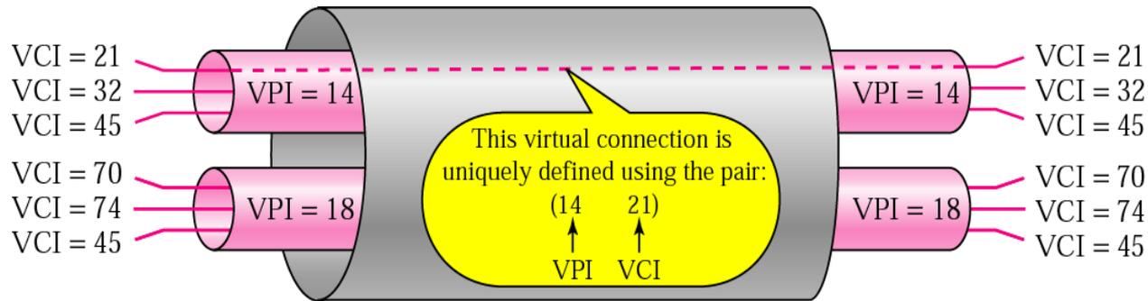
**1- Transmission Path (TP):** the physical connection (wire, cable, satellite, ... ) between an endpoint and a switch or between two switches.
