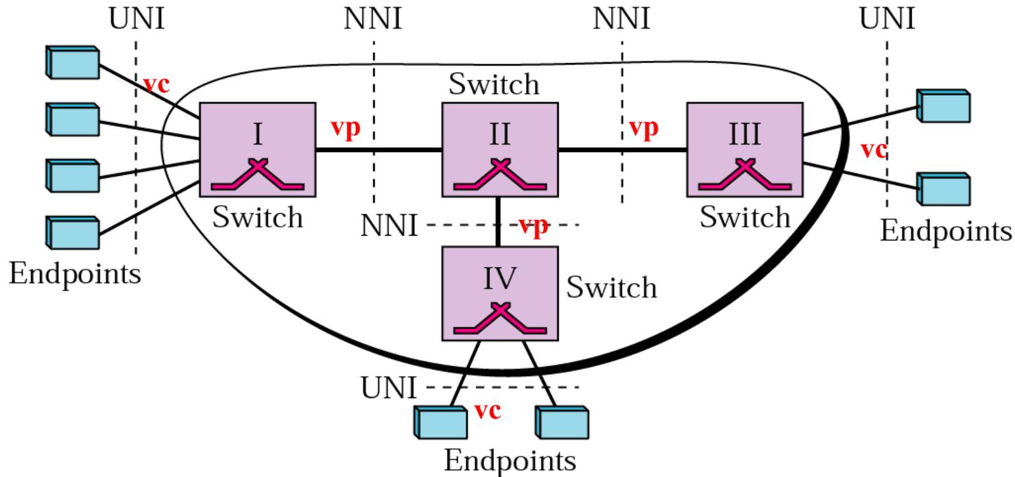
User-to-network interface (**UNI**): interface between endpoint (user access devices) and network switches.
