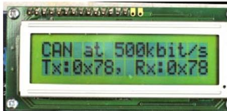
Figure 25 LCD showing CAN frames
