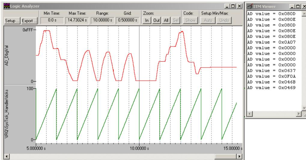
Figure 15 Logic Analyzer and ITM Viewer displaying the variable AD\_DbgVal
