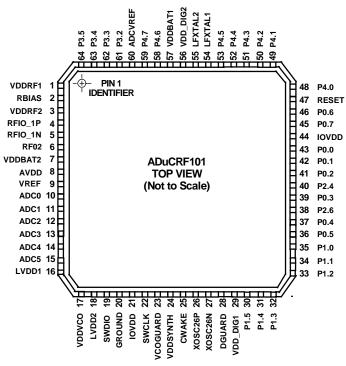
Figure 8. 64-Lead LFCSP\_VQ Pin Configuration
