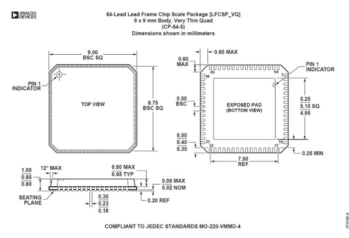
Figure 2. 64-Lead Frame Chip Scale Package [LFCSP\_VQ] 9 mm x 9 mm Body, Very Thin Quad (CP-64-1) Dimensions shown in millimeters
