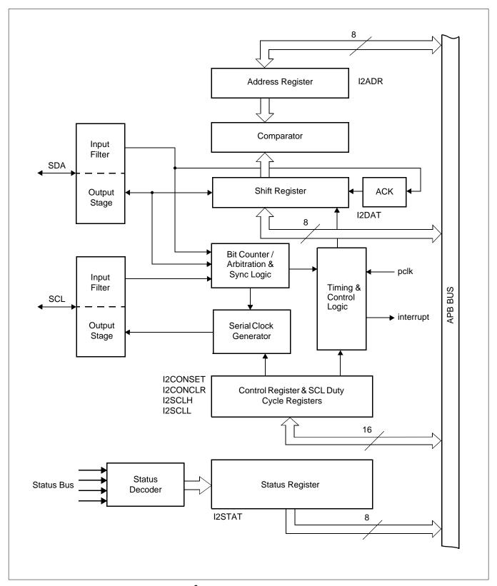
Figure 26: I<sup>2</sup>C Bus Serial Interface Block Diagram
