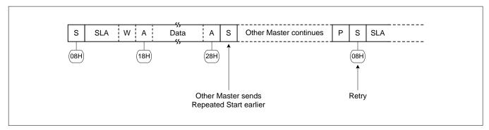
Figure 33: Simultaneous Repeated START Conditions from 2 Masters
