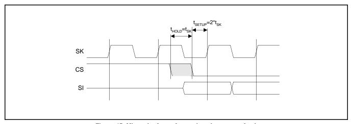
Figure 45: Microwire frame format (continuos transfers)
