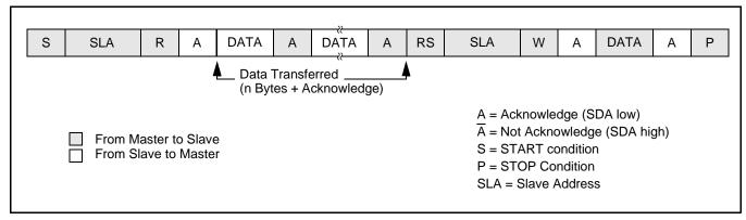
Figure 22: A master receiver switch to master transmitter after sending repeated START
