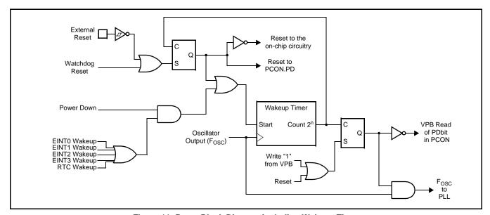
Figure 11: Reset Block Diagram including Wakeup Timer
