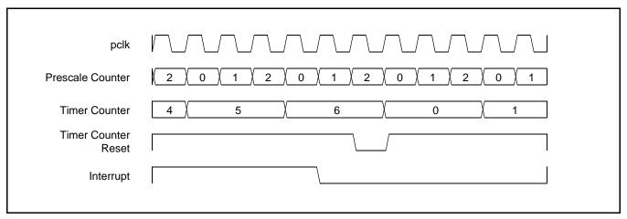
Figure 46: A timer cycle in which PR=2, MRx=6, and both interrupt and reset on match are enabled.
