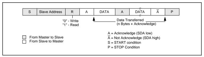
Figure 25: Format of slave transmitter mode
