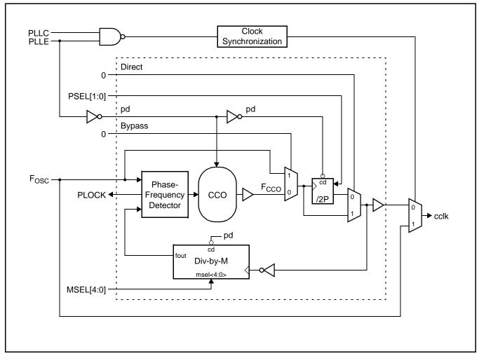
Figure 10: PLL Block Diagram
