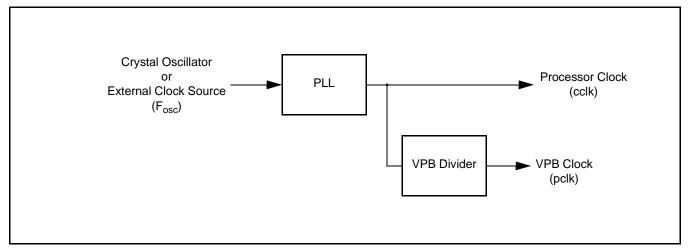
Figure 12: VPB Divider Connections
