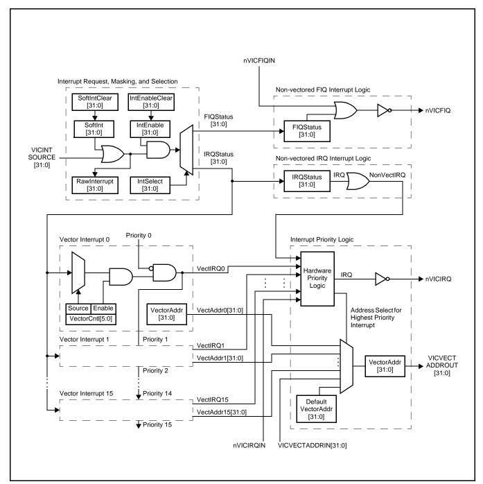
Figure 14: Block Diagram of the Vectored Interrupt Controller
