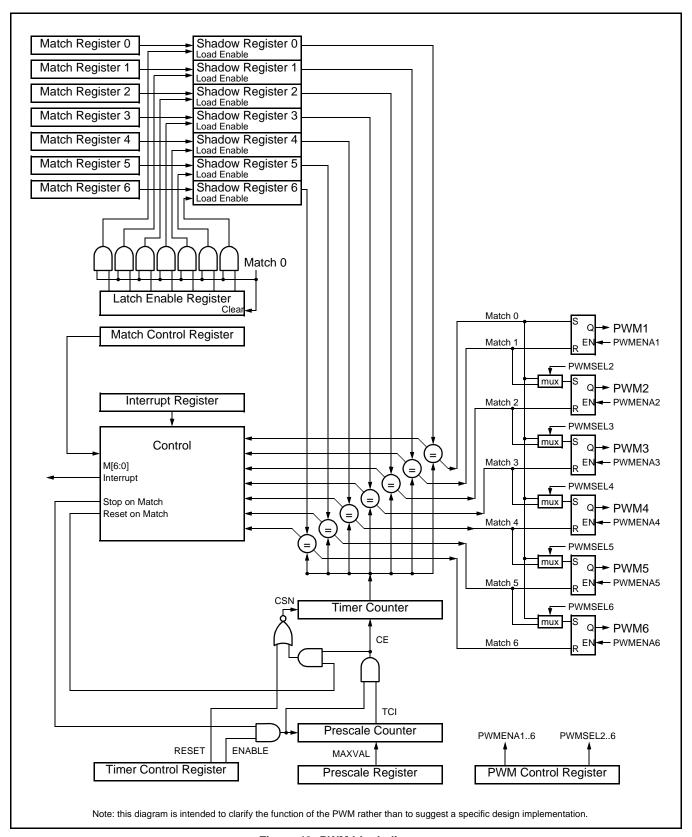
Figure 49: PWM block diagram
