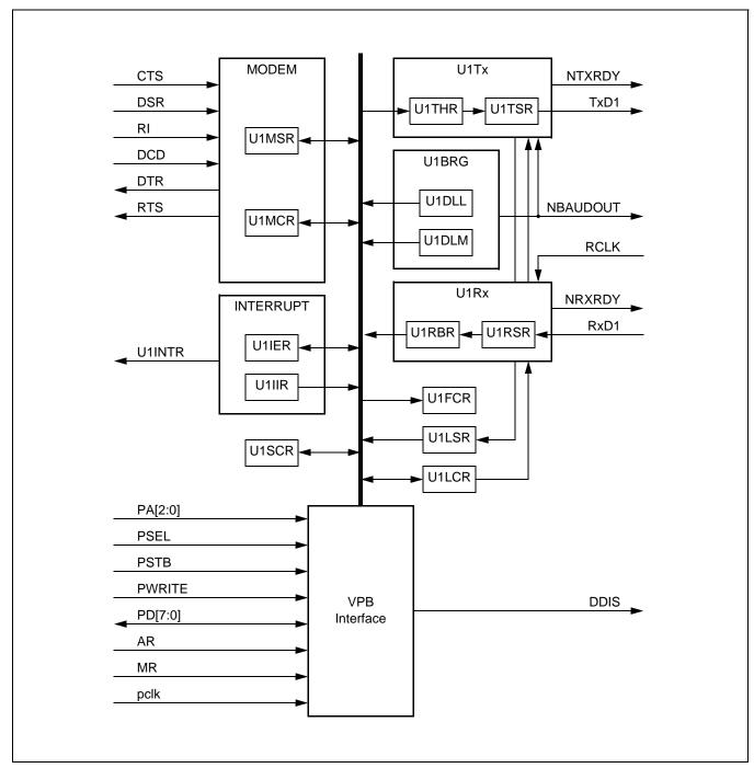
Figure 17: UART1 Block Diagram
