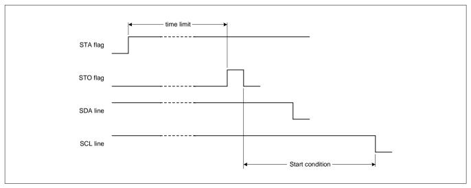
Figure 34: Forced Access to a Busy I<sup>2</sup>C Bus
