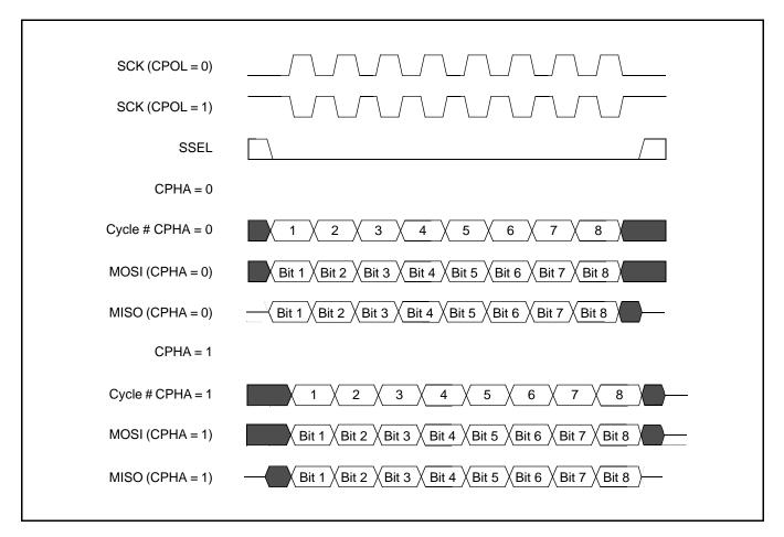
Figure 36: SPI Data Transfer Format (CPHA = 0 and CPHA = 1)
