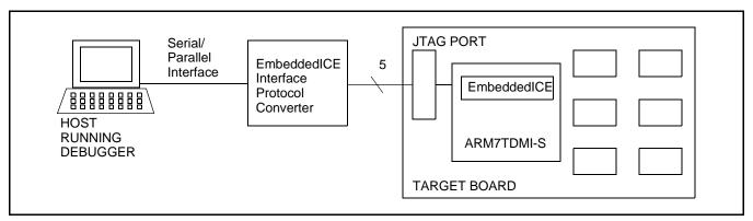
Figure 57: EmbeddedICE Debug Environment Block Diagram
