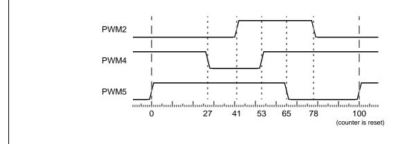
Figure 50: Sample PWM waveforms
