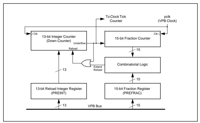
Figure 52: RTC Prescaler block diagram
