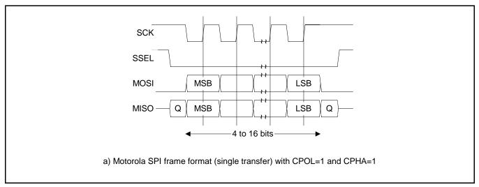
Figure 42: SPI frame format with CPOL=1 and CPHA=1
