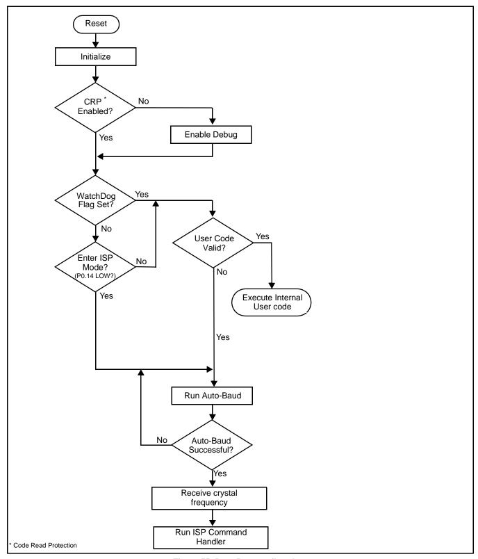
Figure 55: Boot Process flowchart
