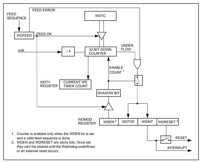
Figure 53: Watchdog Block Diagram
