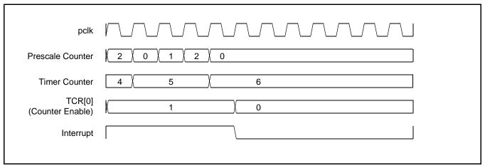
Figure 47: A timer cycle in which PR=2, MRx=6, and both interrupt and stop on match are enabled.
