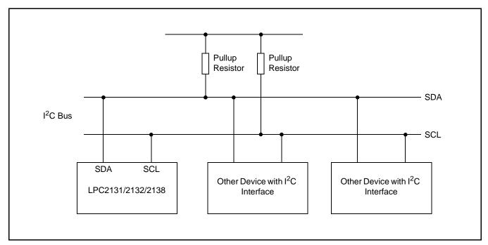
Figure 18: I<sup>2</sup>C Bus Configuration
