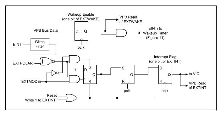
Figure 9: External Interrupt Logic
