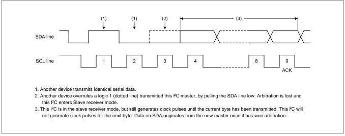
Figure 27: Arbitration Procedure
