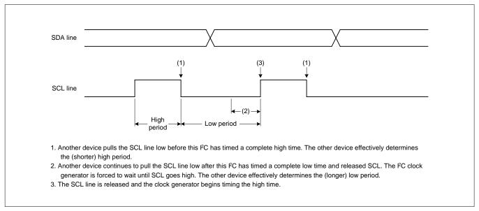
Figure 28: Serial Clock Synchronization (Figure 14)
