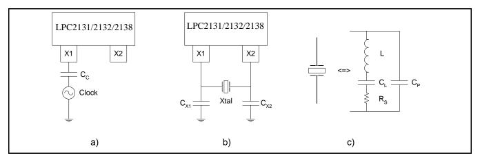
Figure 7: Oscillator modes and models: a) slave mode of operation, b) oscillation mode of operation, c) external crystal model used for C<sub>X1/X2</sub> evaluation
