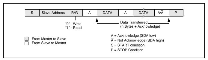
Figure 20: Format in the master transmitter mode
