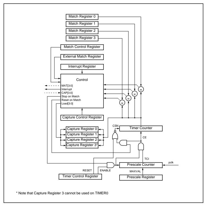
Figure 48: Timer block diagram
