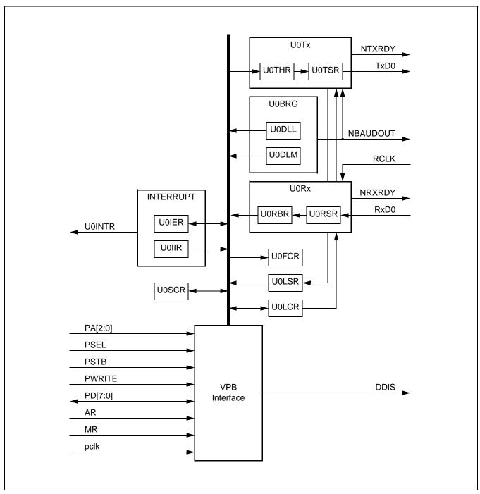
Figure 16: LPC2131/2132/2138 UART0 Block Diagram
