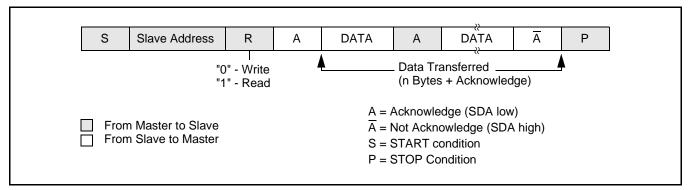
Figure 21: Format of master receiver mode
