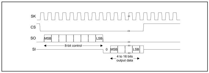
Figure 43: Microwire frame format (single transfer)
