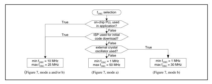
Figure 8: F<sub>OSC</sub> selection algorithm
