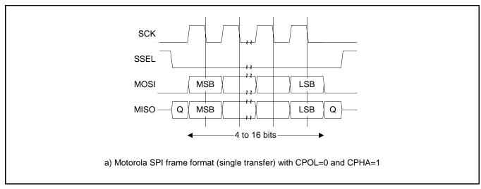
Figure 40: SPI frame format with CPOL=0 and CPHA=1
