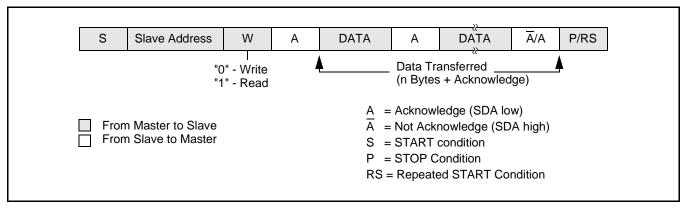
Figure 24: Format of slave receiver mode
