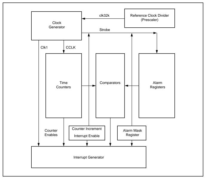
Figure 51: RTC block diagram
