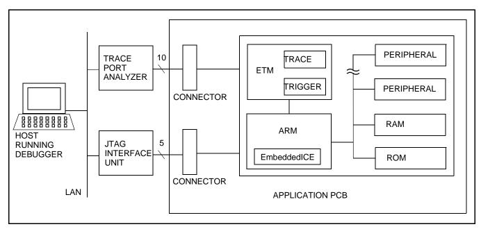
Figure 58: ETM Debug Environment Block Diagram
