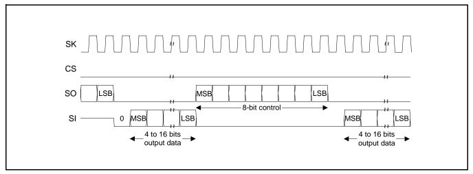
Figure 44: Microwire frame format (continuos transfers)
