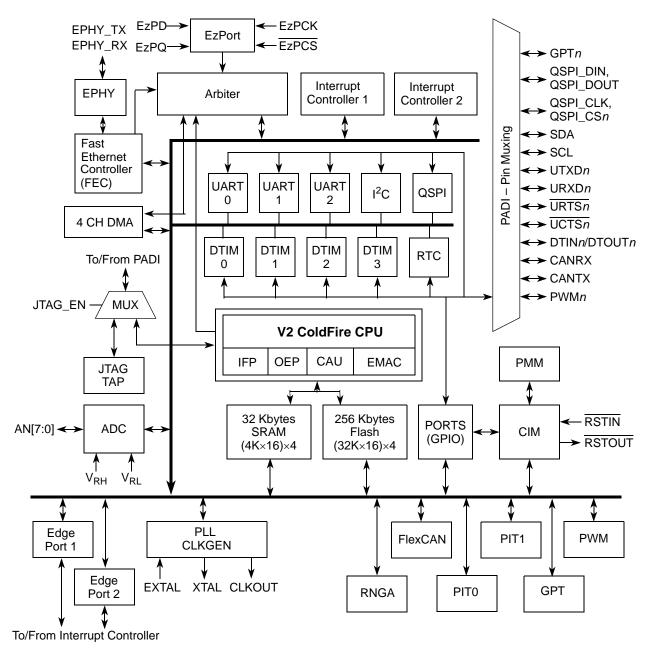
Figure 1. MCF52235 Block Diagram
