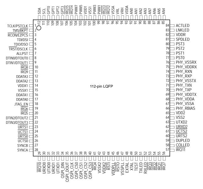
Figure 3. 112-pin LQFP Pin Assignments
