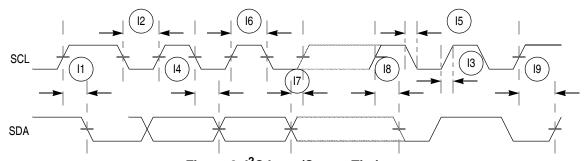
Figure 8. I<sup>2</sup>C Input/Output Timings
