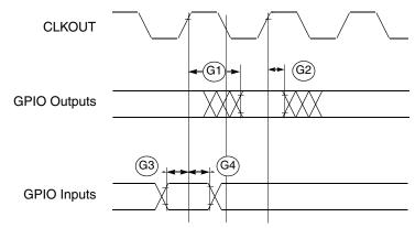
Figure 6. GPIO Timing
