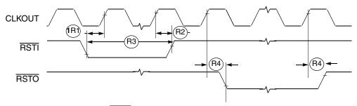
Figure 7. RSTI and Configuration Override Timing
