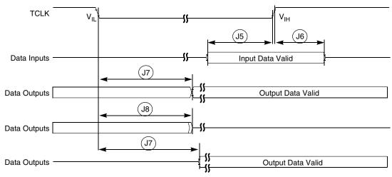
Figure 13. Boundary Scan (JTAG) Timing
