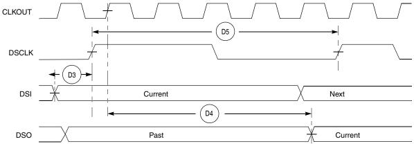
Figure 17. BDM Serial Port AC Timing
