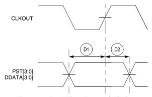
Figure 16. Real-Time Trace AC Timing
