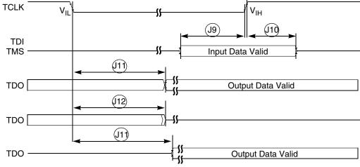
**Figure 14. Test Access Port Timing**
