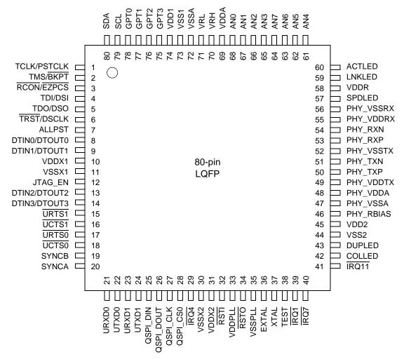
Figure 2. 80-pin LQFP Pin Assignments
