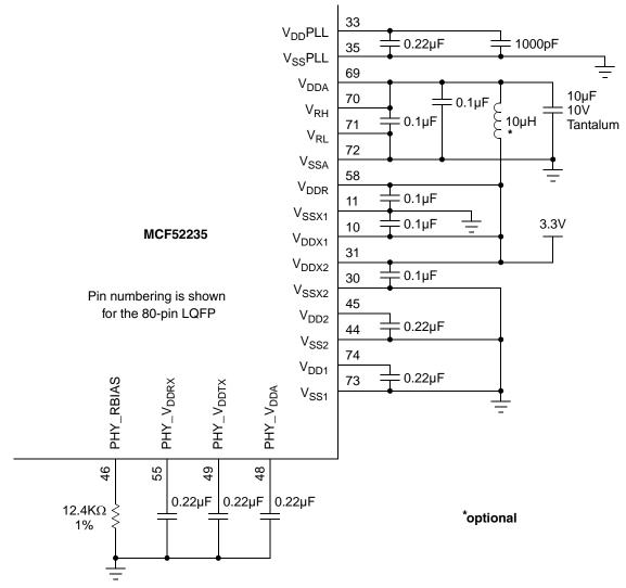
Figure 5. Suggested Connection Scheme for Power and Ground
