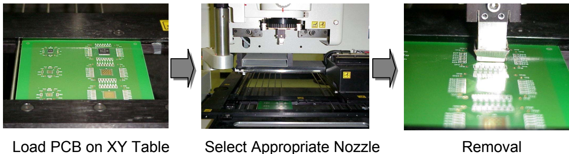
Figure 24. Package Removal Process
