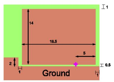
Figure 26. Patch Antenna 1
