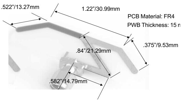
Figure 19. Dipole Antenna With Dimensions
