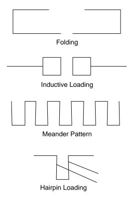
Figure 3. Dipole Loading Examples
