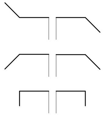
Figure 2. Dipole Shapes to Improve Omnidirectional Characteristics
