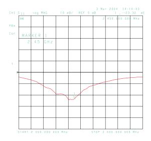
Figure 16. F Antenna Return Loss and Bandwidth
