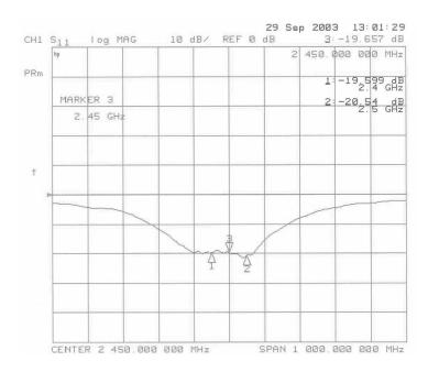
Figure 20. VSWR Plot of Dipole Antenna
