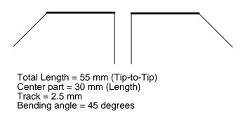
Figure 18. Single Bend Dipole
