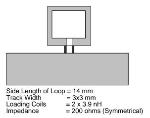
Figure 24. Experimental Full Wave Loop
