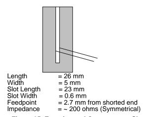
Figure 25. Experimental Quarter-wave Slot
