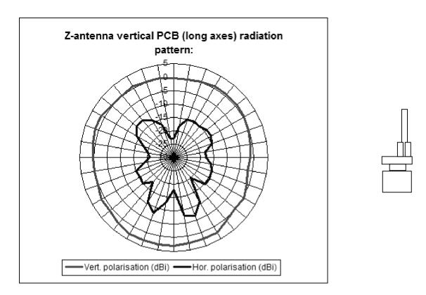
Figure 22. Antenna Pattern for Dipole Antenna in Position Shown (2 of 3)
