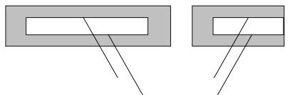
Figure 10. Half-wave and Quarter-wave Slot Antennas
