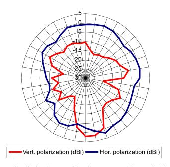
Figure 14. F-Antenna Radiation Pattern (For Antennas as Shown in Figures 11 and 12)
