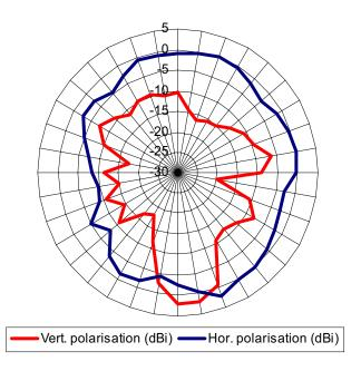
Figure 15. F-Antenna Radiation Pattern (Rotated 90 Degrees For Antennas as Shown in Figures 11 and 12)
