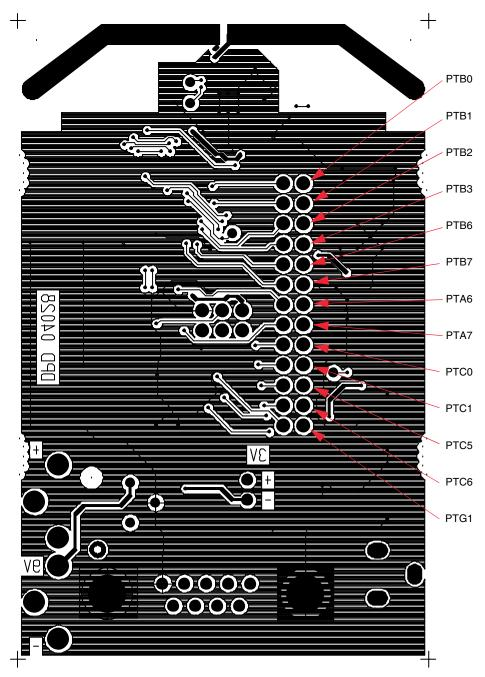
Figure A-2. PCB Layout (Bottom View)
