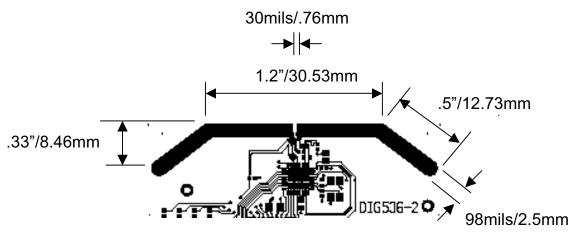
Figure A-3. Printed Circuit Board Antenna Dimensions
