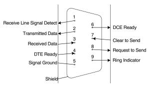
Figure 1-3. DCE-DB9 Female Connector (Looking into the SARD Connector)
