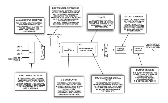
Figure 8. Auxiliary ADC Block Diagram
