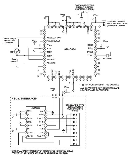
Figure 66. Typical System Configuration
