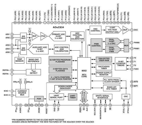
Figure 1. Detailed Block Diagram
