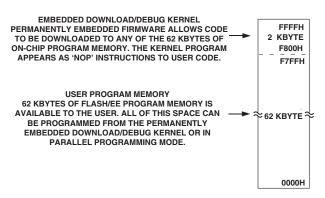
Figure 17. Flash/EE Program Memory Map in Normal Mode
