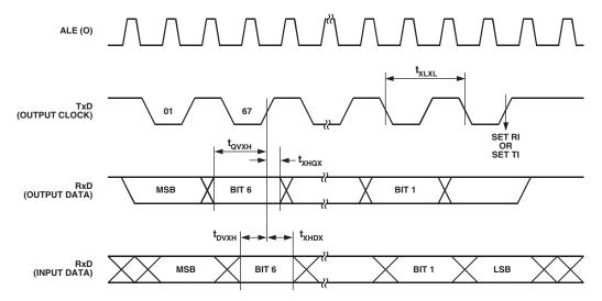
Figure 74. UART Timing in Shift Register Mode
