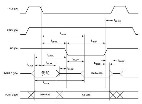
Figure 72. External Data Memory Read Cycle
