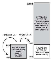
Figure 4. Extended Stack Pointer Operation
