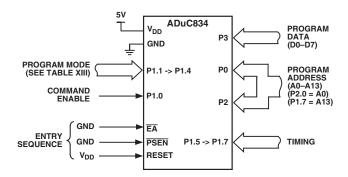
Figure 18. Flash/EE Memory Parallel Programming
