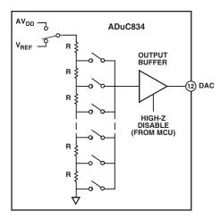
Figure 21. Resistor String DAC Functional Equivalent
