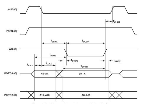
Figure 73. External Data Memory Write Cycle
