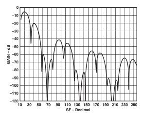
Figure 14. 60 Hz Normal Mode Rejection vs. SF
