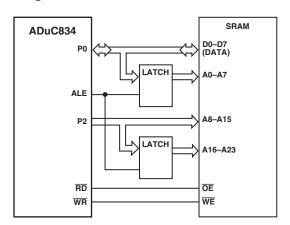
Figure 60. External Data Memory Interface (16 Mbytes Address Space)
