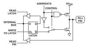
Figure 36. Port 0 Bit Latch and I/O Buffer
