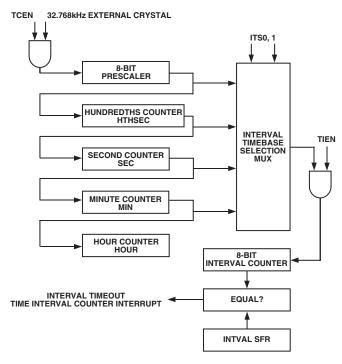
Figure 33. TIC, Simplified Block Diagram
