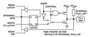
Figure 40. Port 2 Bit Latch and I/O Buffer
