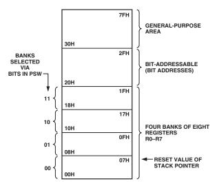
Figure 2. Lower 128 Bytes of Internal Data Memory
