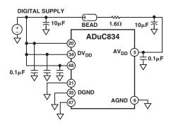
Figure 62. External Single Supply Connections
