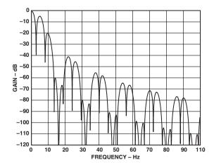
Figure 12. Filter Response, SF = 255 dec
