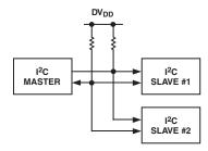
Figure 35. Typical I<sup>2</sup>C System
