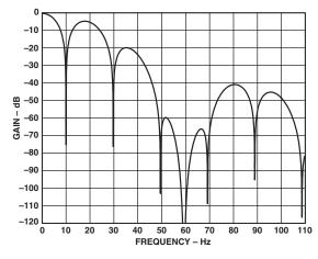
Figure 11. Filter Response, SF = 69 dec
