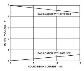
Figure 23. Source and Sink Current Capability with  $V_{REF} = AV_{DD} = 5 V$
