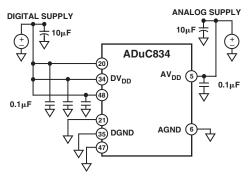
Figure 61. External Dual Supply Connections
