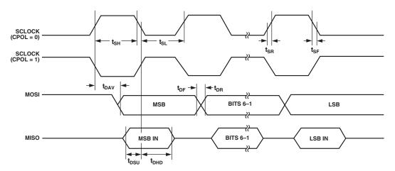
Figure 76. SPI Master Mode Timing (CPHA = 0)
