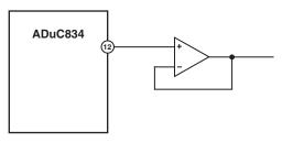
Figure 25. Buffering the DAC Output
