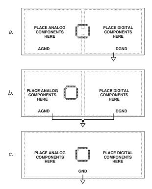
Figure 64. System Grounding Schemes
