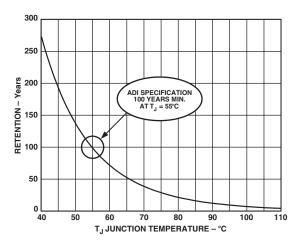
Figure 16. Flash/EE Memory Data Retention
