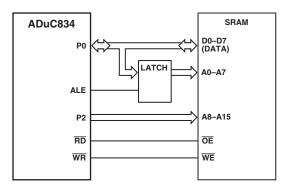
Figure 59. External Data Memory Interface (64 Kbytes Address Space)
