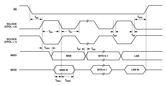
Figure 77. SPI Slave Mode Timing (CPHA = 1)
