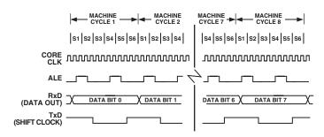
Figure 54. UART Serial Port Transmission, Mode 0
