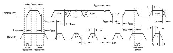
Figure 79. I<sup>2</sup>C Compatible Interface Timing
