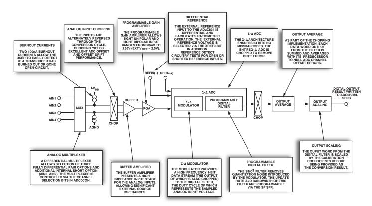
Figure 7. Primary ADC Block Diagram
