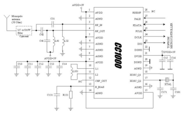
Figure 2. Typical CC1000 application circuit
