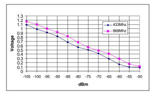
Figure 14. RSSI voltage vs. input power
