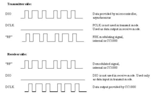
Figure 9. Transparent Asynchronous UART mode
