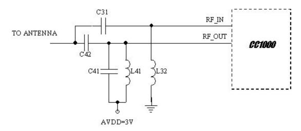
Figure 12. Input/output matching network
