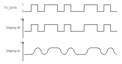
Figure 17. FSK spectrum shaping by smooth frequency transitions
