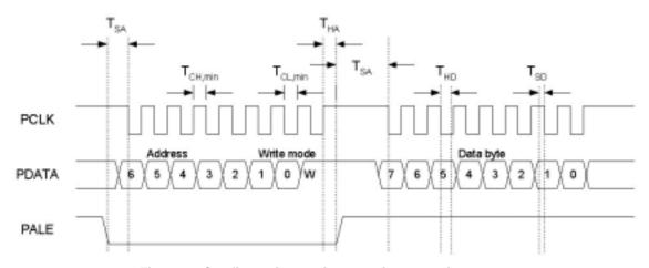
Figure 4. Configuration registers write operation
