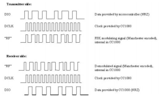
Figure 8. Synchronous Manchester encoded mode
