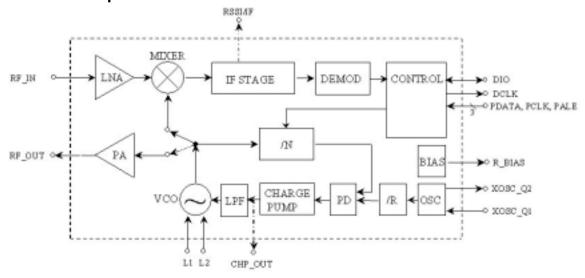
Figure 1. Simplified block diagram of the CC1000.
