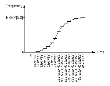
Figure 18. Stepwise frequency shaping
