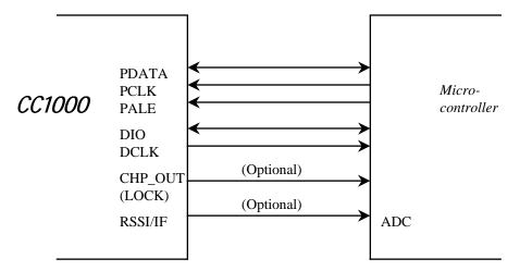
Figure 6. Microcontroller interface
