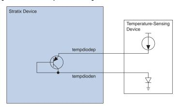
Figure 79. External Temperature-Sensing Diode
