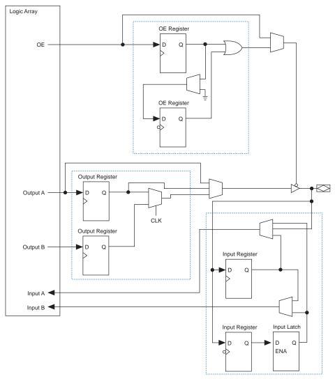
The IOEs are located in I/O blocks around the periphery of the Stratix device. There are up to four IOEs per row I/O block and six IOEs per column I/O block. The row I/O blocks drive row, column, or direct link interconnects. The column I/O blocks drive column interconnects. Figure 59 shows how a row I/O block connects to the logic array. Figure 60 shows how a column I/O block connects to the logic array.
