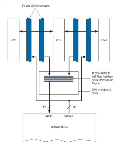
Figure 23. M-RAM Column Unit Interface to Interconnect
