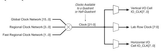
IOE clocks have horizontal and vertical block regions that are clocked by eight I/O clock signals chosen from the 22 quadrant or half-quadrant clock resources. Figures 47 and 48 show the quadrant and half-quadrant relationship to the I/O clock regions, respectively. The vertical regions (column pins) have less clock delay than the horizontal regions (row pins).
