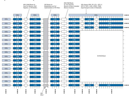
The number of M512 RAM, M4K RAM, and DSP blocks varies by device along with row and column numbers and M-RAM blocks. Table 6 lists the resources available in Stratix devices.
