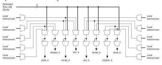
Figure 18. M4K RAM Block LAB Row Interface
