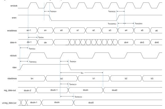
Figure 81. Dual-Port RAM Timing Microparameter Waveform
