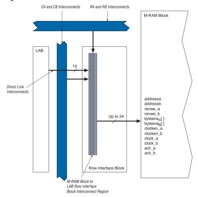
Figure 22. M-RAM Row Unit Interface to Interconnect
