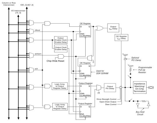
Figure 65. Stratix IOE in DDR Output I/O Configuration Note (1)
