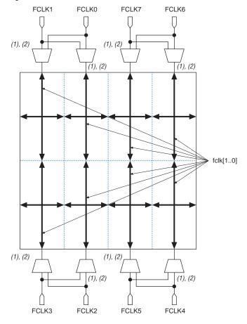
Figure 45. EP1S120 to EP1S30 Device Fast Regional Clock Pin Connections to Fast Regional Clocks
