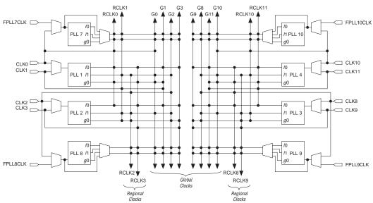
Figure 50. Global & Regional Clock Connections from Side Pins & Fast PLL Outputs Note (1)
