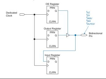
All external I/O timing parameters shown are for 3.3-V LVTTL I/O standard with the maximum current strength and fast slew rate. For external I/O timing using standards other than LVTTL or for different current strengths, use the I/O standard input and output delay adders in Tables 116 through 118.
