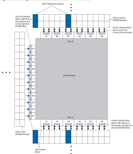
Figure 21. Left-Facing M-RAM to Interconnect Interface Notes (1), (2)
