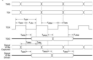
Figure 75. Stratix JTAG Waveforms
