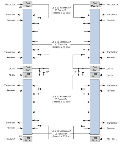
Figure 74. Fast PLL & Channel Layout in the EP1S30 to EP1S120 Devices
