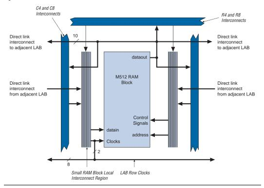
Figure 16. M512 RAM Block LAB Row Interface
