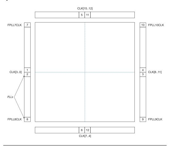
Figure 50 shows the global and regional clocking from the PLL outputs and the CLK pins.
