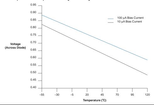
Figure 80. Temperature vs. Temperature-Sensing Diode Voltage
