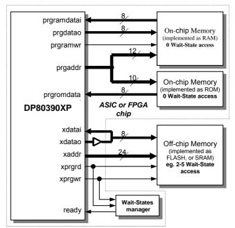
The described above implementation should be treated as an example. All Program Memory spaces are fully configurable. For timing-critical applications whole program code can be implemented as on-chip ROM and (or) RAM and executed without Wait-States, but for some other applications whole program code can be implemented as off-chip ROM or FLASH and executed with required number Wait-State cycles.
