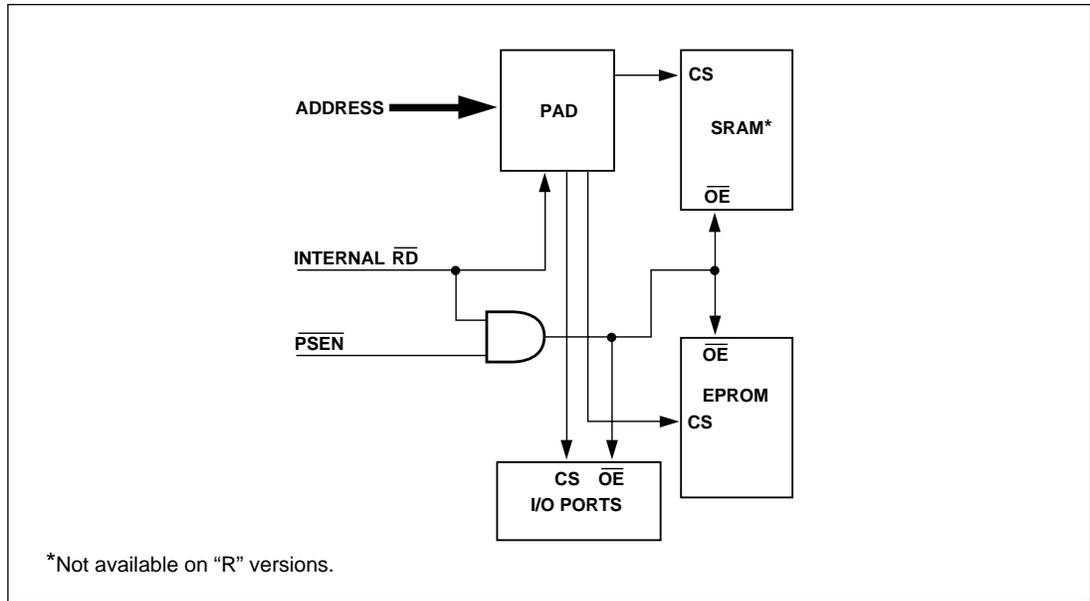
**Figure 10. 8031-Compatible Separate Code and Data Address Spaces**
