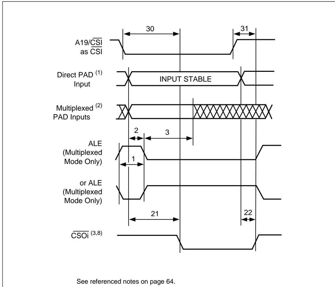
Figure 37. Port A as AD0–AD7 Timing (Track Mode) Using  $\overline{RD}$ ,  $\overline{WR}$  (PSD3X1)
