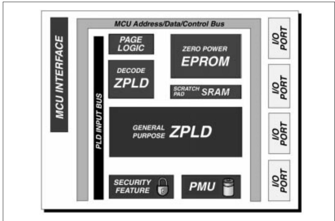
The PSD3XX family architecture (Figure 1) can efficiently interface with, and enhance, almost any 8- or 16-bit microcontroller system. This solution provides microcontrollers the following:
