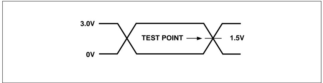
Figure 41B. AC Testing Input/Output Waveform (3 V Versions)
