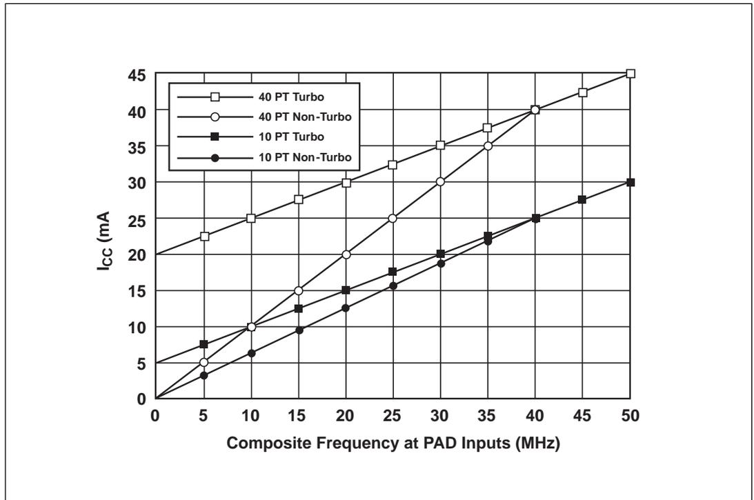
**Figure 15. Typical  $I_{CC}$  vs. Frequency ( $V_{CC} = 3\text{ V}$ )**
