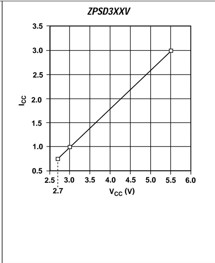
Figure 18. Normalized  $I_{CC}$  (AC) ( $V_{CC} = 3.0\text{ V}$ )
