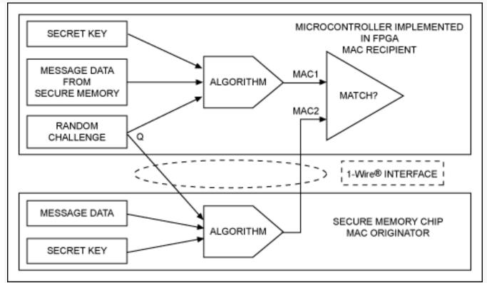
Figure 1. The challenge-and-response authentication process proves the authenticity of a MAC originator.
