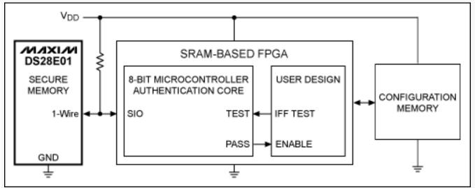
Figure 2. In this simplified schematic, a secure 1-Wire memory is used for FPGA protection.
