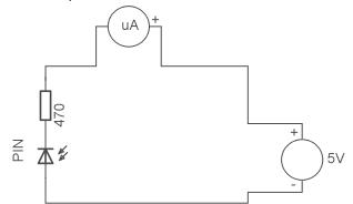
4. Connect the **phototransistor**, milliammeter and power supply to the breadboard according to the schematics below. The phottransistor is directional, make sure it is pointed to the light source. Place the reference luxmeter as close to DUT as possible, cover the assembly with
