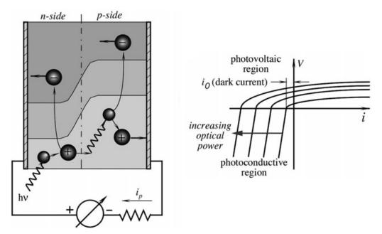
Depending on external polarization of the junction, these pairs create a photovoltage (open circuit) or photocurrent (reverse polarization). Created photo signal ceases once one charge carrier of the created electron-hole pair recombinates. As a result, photoelectric sensors are much faster than photoconductors. Ideal photodiode has no dark current and thus is better suited for low intensity light measurement.
