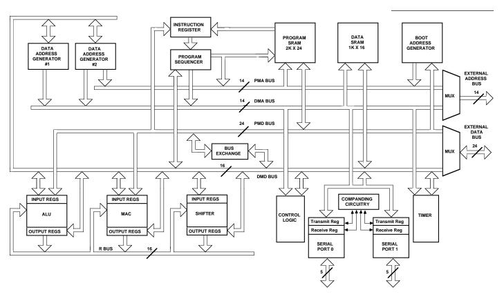
Figure 1.3 ADSP-2101 Internal Architecture
