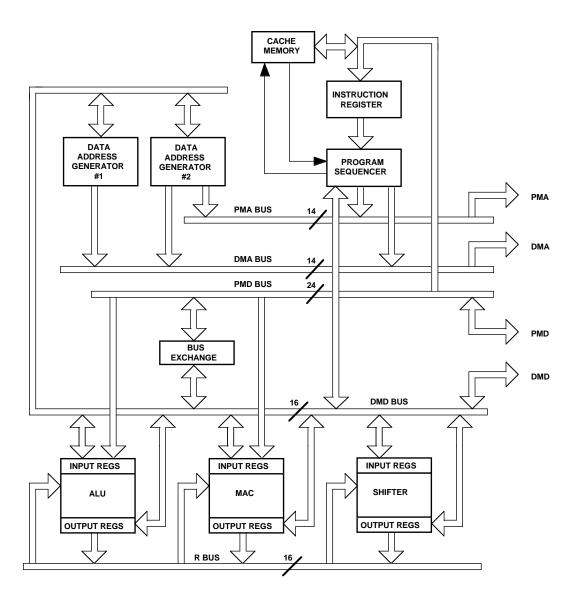
Figure 1.1 ADSP-2100 Internal Architecture
