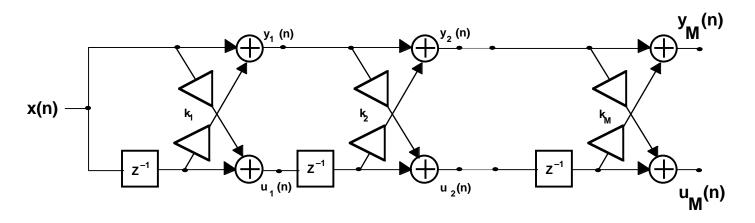
Figure 5.3 All-Zero Lattice Filter
