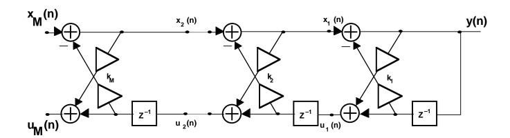
Figure 5.4 All-Pole Lattice Filter Structure
