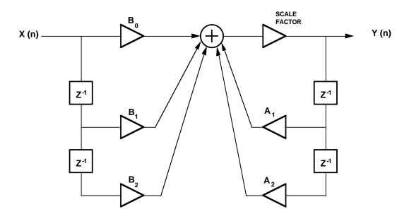
Figure 5.2 Second-order Biquad IIR Filter Section
