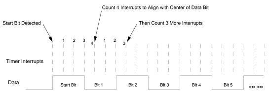
Figure 11.3 Receive Data Timing
