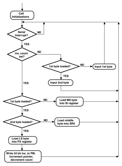
Figure 12.8 Boot Program Flow Diagram
