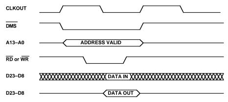
Figure 12.2 DSP Read/Write Timing
