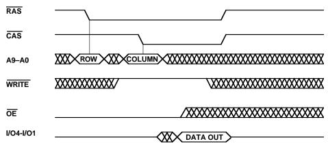
Figure 12.3 DRAM Read Cycle Timing
