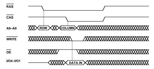
Figure 12.4 DRAM Delayed-Write (Output Enabled) Cycle Timing
