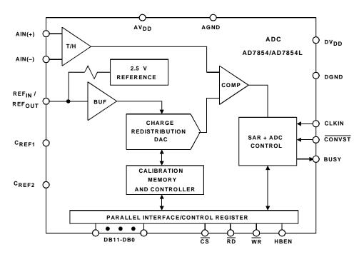
Figure 10-3. AD7854/AD7854L Functional Block Diagram
