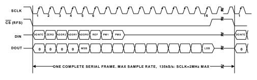
Figure 10-24. ADSP-218x DSP to AD7888 ADC Serial Interface Timing
