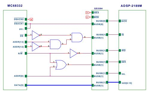
Figure 10-30. Glue Logic between the MC68332 and the ADSP-2189M Using Address Decoding
