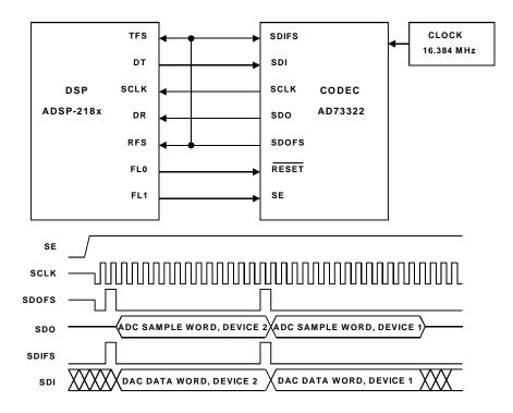
Figure 10-17. AD73322 Interface to ADSP-218x Family Processors
