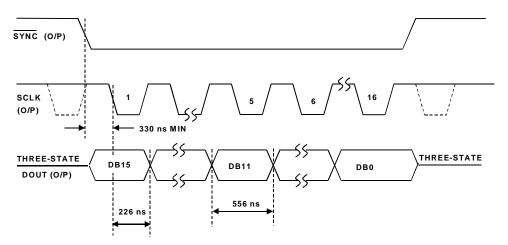
Figure 10-12. AD7853L ADC Serial Output Timing
