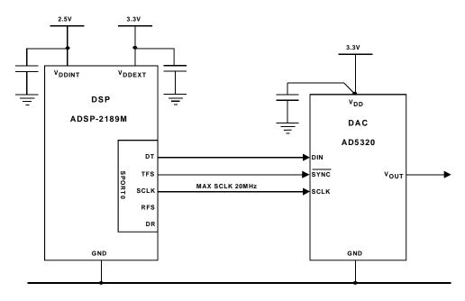
Figure 10-26. ADSP-218x DSP to AD5320 DAC Serial Interface
