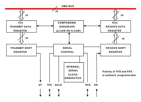
Figure 10-9. ADSP-218x Family Serial Port Block Diagram
