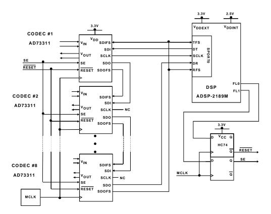
Figure 10-20. AD7311 Codec(s) to ADSP-218x DSP Serial Interface
