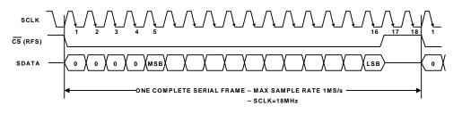
Figure 10-22. ADSP-218x DSP to AD7475/95 ADC Serial Interface Timing
