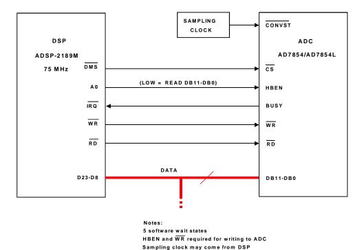
Figure 10-4. AD7854/AD7854L ADC Parallel Interface to ADSP-2189M
