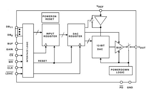
Figure 10-7. AD5340 Parallel Input DAC
