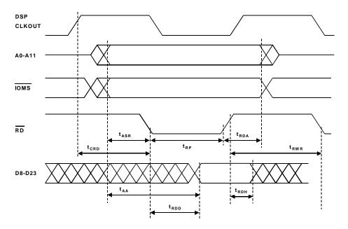
Figure 10-2 shows the timing diagram for the ADSP-218x read-cycle.
