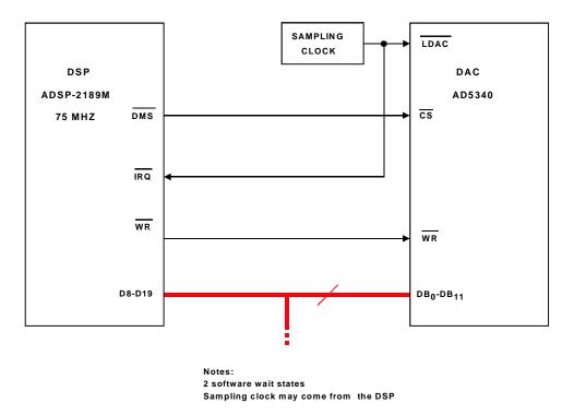
Figure 10-8. AD5340 DAC Parallel Interface to ADSP-2189M
