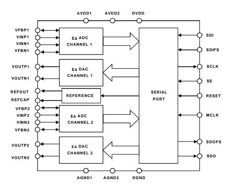
Figure 10-16 shows a functional block diagram of the AD73322.
