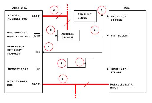
Figure 10-5. DAC to ADSP-218x DSP Parallel Interface
