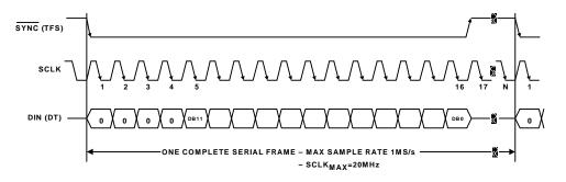
Figure 10-27. ADSP-218x DSP to AD5320 DAC Serial Interface Timing
