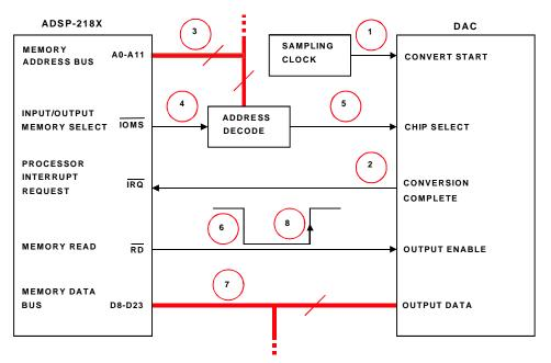
Figure 10-1. ADC to ADSP-218x DSP Parallel Interface
