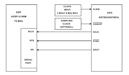
Figure 10-13. AD7853/AD7853L ADC Serial Interface to ADSP-2189M
