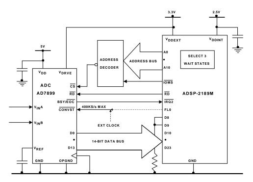
Figure 10-25. ADSP-218x DSP to AD7899 ADC Parallel Interface
