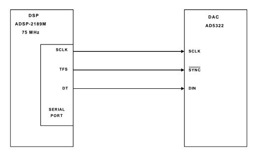
Figure 10-15. AD5322 DAC Serial Interface to ADSP-2189M
