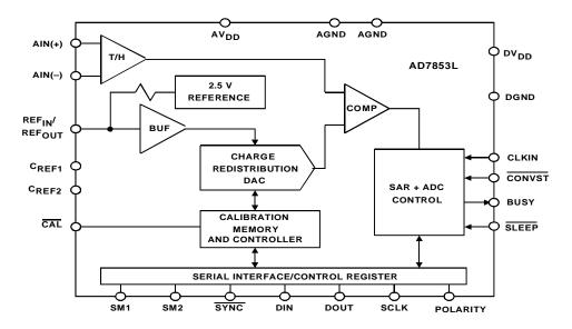
Figure 10-11 shows a block diagram of the AD7853/AD7853L.
