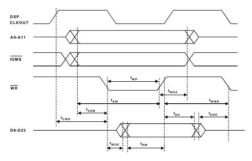
Figure 10-6 shows the memory-write cycle timing diagram for the ADSP-21xx-family.
