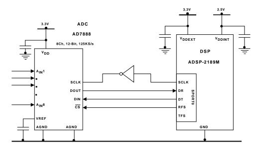
Figure 10-23. ADSP-218x DSP to AD7888 ADC Serial Interface
