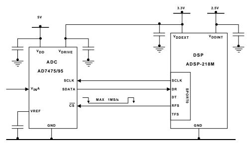
Figure 10-21. ADSP-218x DSP to AD7475/95 ADC Serial Interface
