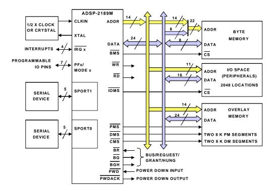
Figure 10-19. ADSP-2189M System Interface (Full Memory Mode)
