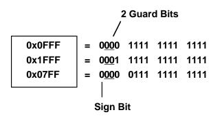
To detect bit growth into 2 guard bits, set SB=–2 Figure C.4 Data With Guard Bits
