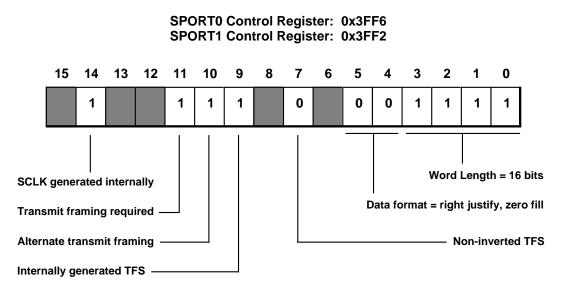
Figure 13.5 SPORT To AD766 DAC Control Register Settings
