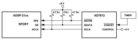
Figure 13.6 Serial Port Interface To AD7872 ADC
