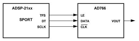
Figure 13.3 Serial Port Interface To AD766 DAC
