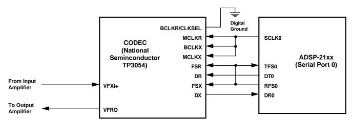
Figure 13.2 ADSP-21xx Serial Port (SPORT0) To CODEC
