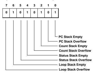
Figure 3.5 SSTAT Register (Read-Only)
