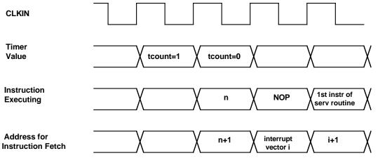
Figure 3.3 Timer Interrupt Latency for ADSP-2101, ADSP-2105, ADSP-2115, ADSP-2111 3 - 19
