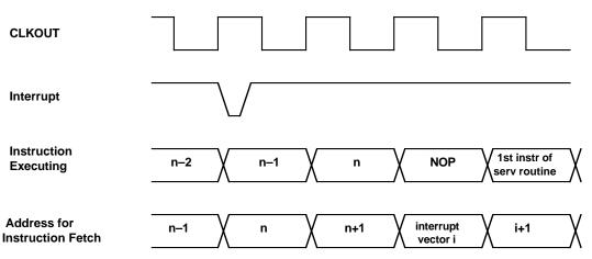
Figure 3.2 Interrupt Latency (Timer, IROx, SPORT, HIP, & Analog Interrupts)
