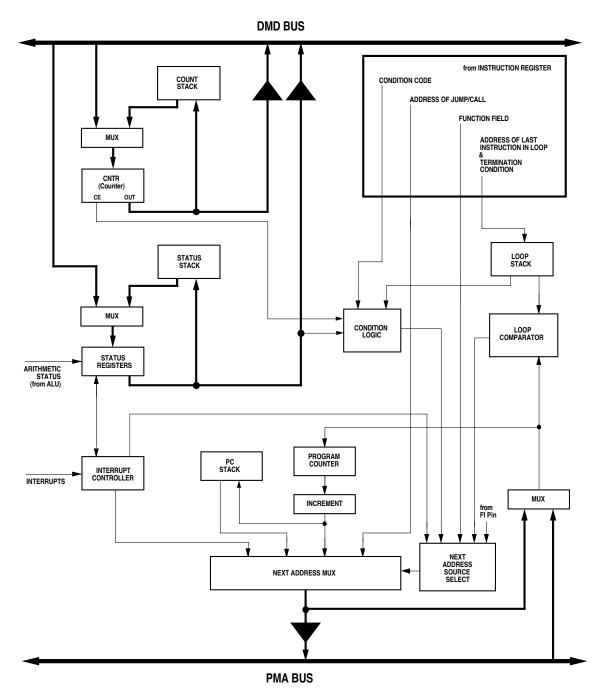
Figure 3.1 Program Sequencer Block Diagram
