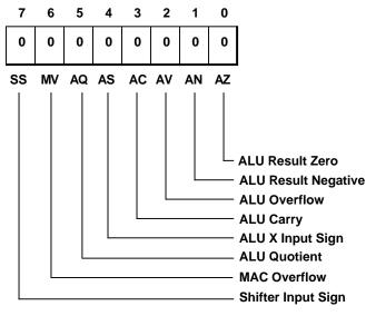
Each of the bits is automatically updated when a new status is generated by an arithmetic instruction. Each bit is affected only by a subset of arithmetic operations, as defined by the following table:
