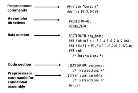
Figure 1-2. Assembly Code File Structure for SHARC Processors
