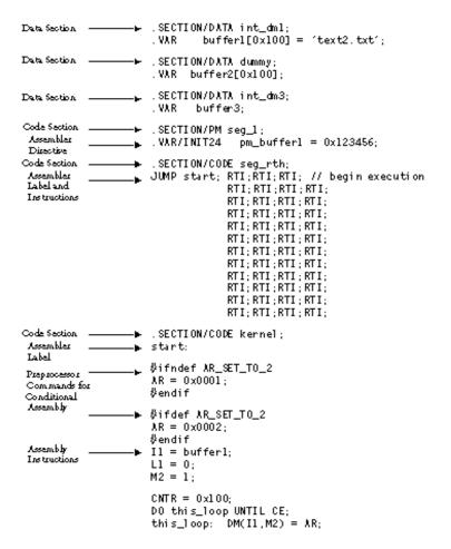
Figure 1-4. Assembly Source File Structure for Blackfin Processors
