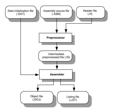
Figure 1-1. Assembler Input and Output Files
