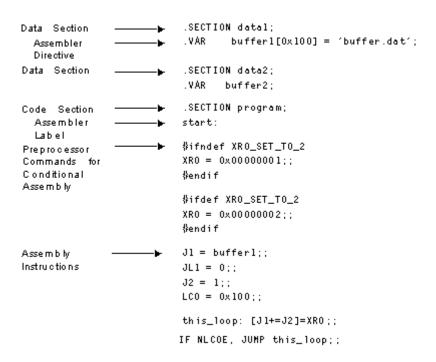
Figure 1-3. Assembly Code File Structure for TigerSHARC Processors
