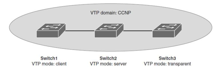
Step 1. Configure VTP on all the switches, Switch 1 and Switch 3 as client mode where as Switch2 as server mode
